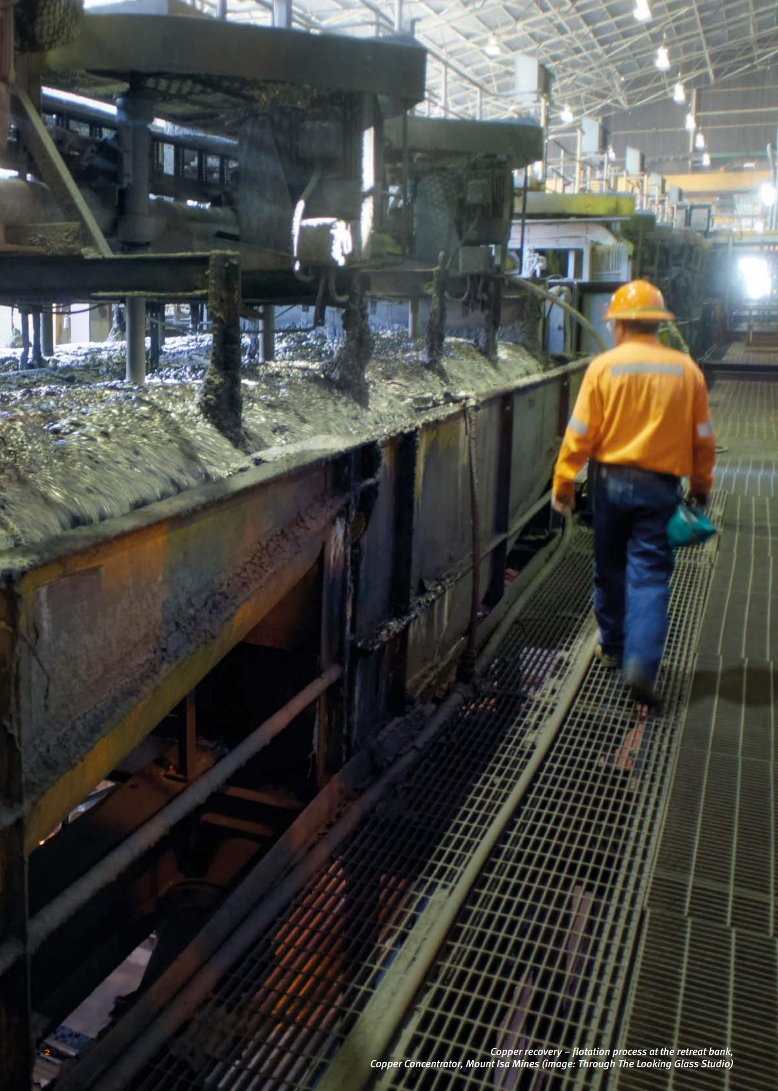
*Copper recovery – flotation process at the retreat bank, Copper Concentrator, Mount Isa Mines (image: Through The Looking Glass Studio)*
