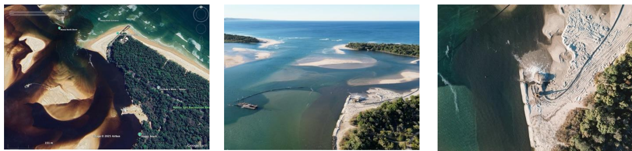
Figure 9: Left: Aerial image of Noosa dog beach (Google Earth, 2024), Middle and Right: Drone images of sand being pumped from inner channel to create closure of nearshore channel (ICM, 2024)
