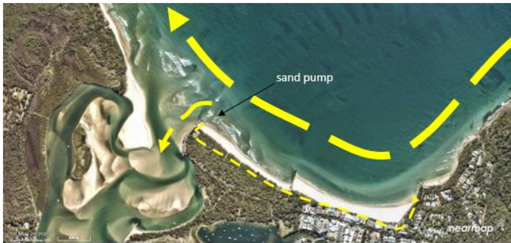
Figure 14: Aerial image of Noosa Backpass / Bypass System (small, dotted lines) (Jackson, 2023)
