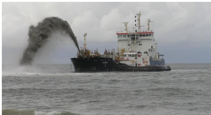
Figure 5: Photo of "Brisbane" rainbowing nourishment into the nearshore zone of Woorim beach
