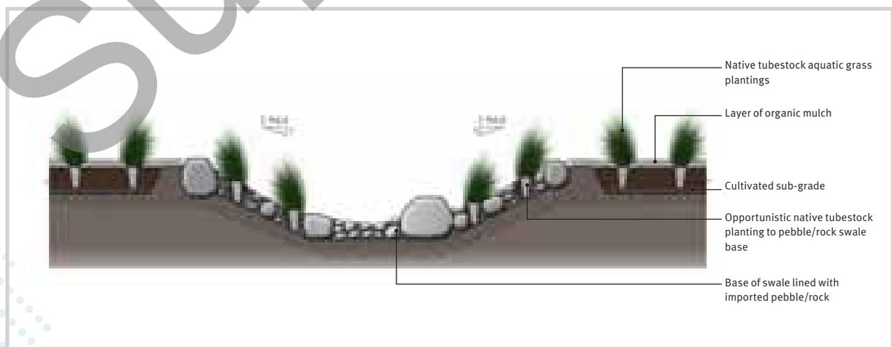
Typical section of rock-lined and vegetated swale
