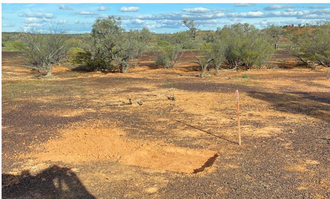
**Plate 3.3 Example of a CSEM Electrode Pit**
