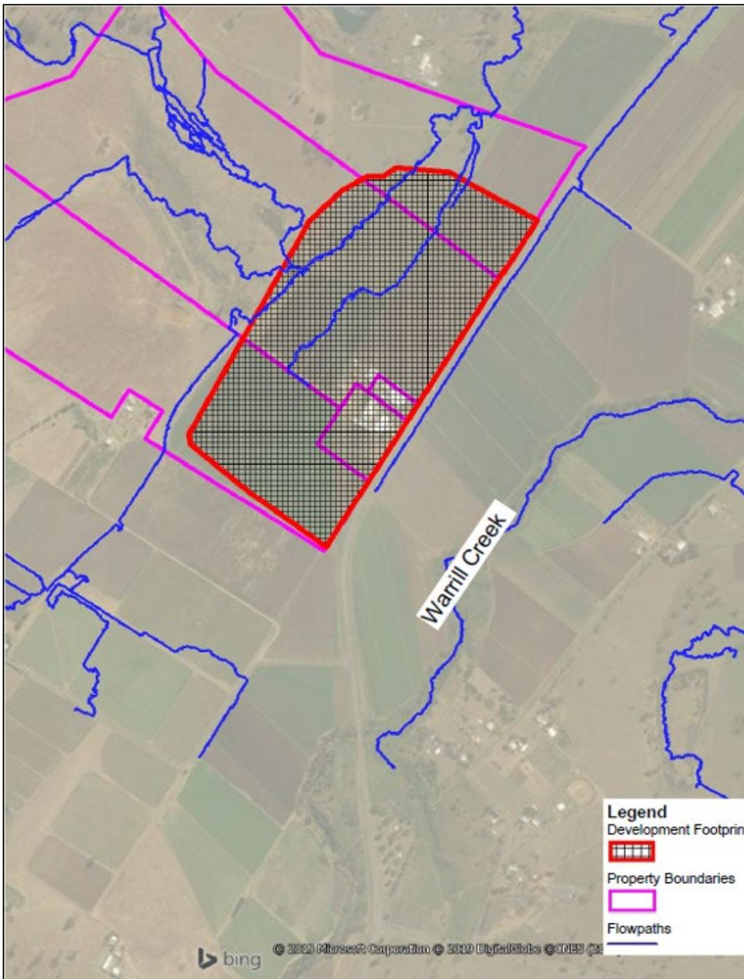
The site is located on a floodplain that is inundated by Warrill Creek. Additional to the Warrill Creek flooding there are two catchments located to the West of the site, draining along the western boundary of the development area.
