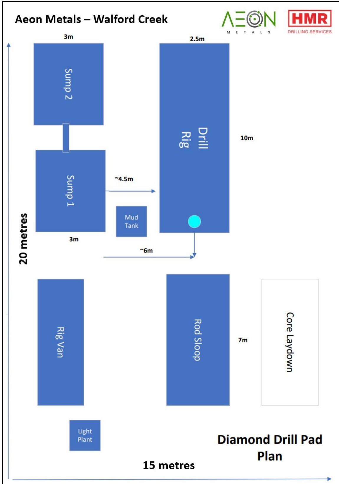
Figure 2 Schematic of the Proposed Drill Pad
