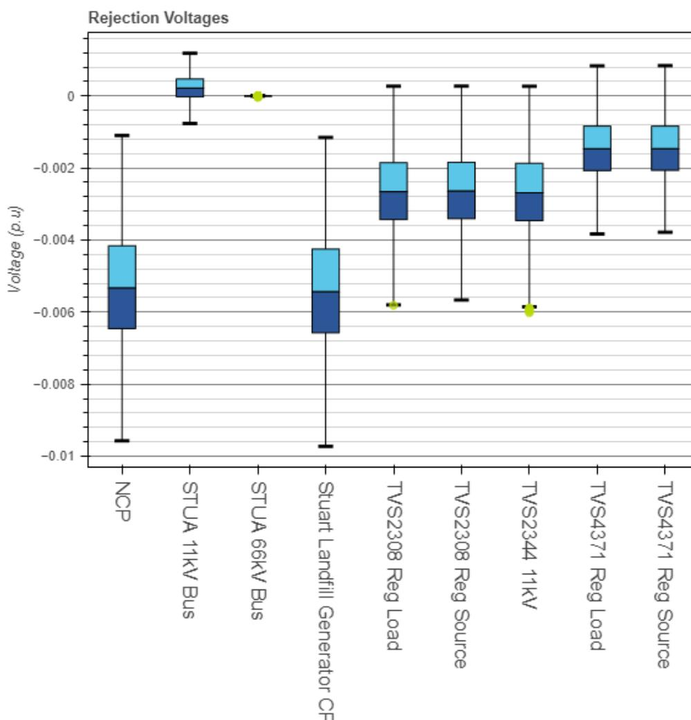
Figure 25- Voltage Step on Loss of Generation
