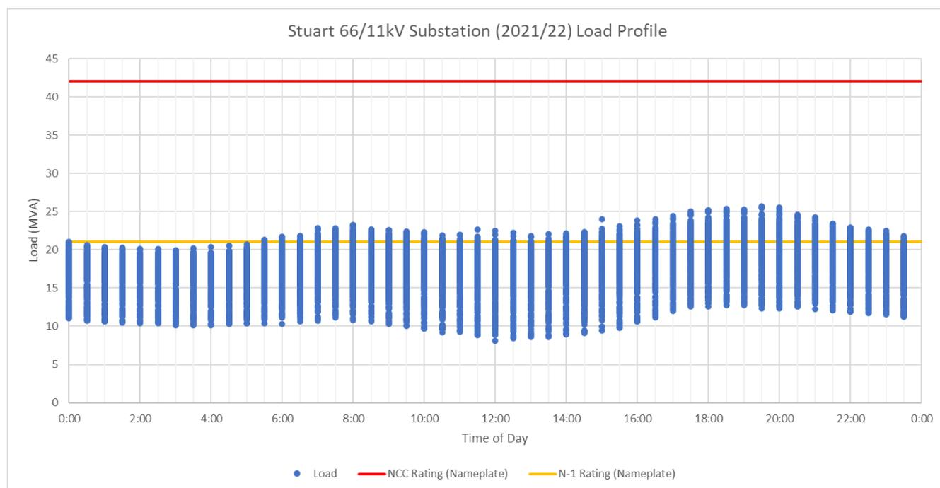
**Figure 4 – Stuart Substation Load Profile**
