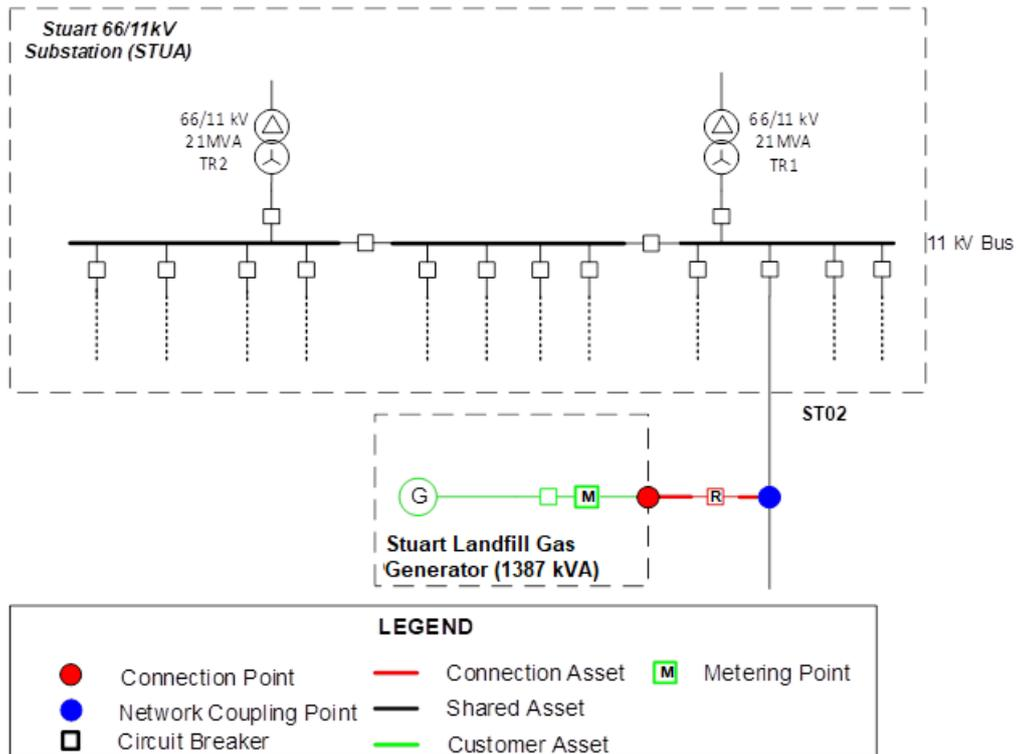
Figure 27 - Single Line diagram of Option 1
