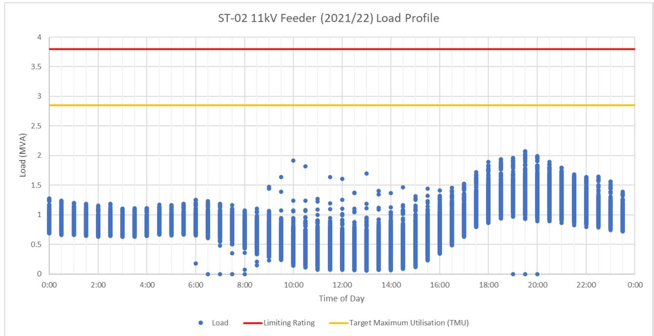
**Figure 5 – ST-02 Feeder Load Profile**
