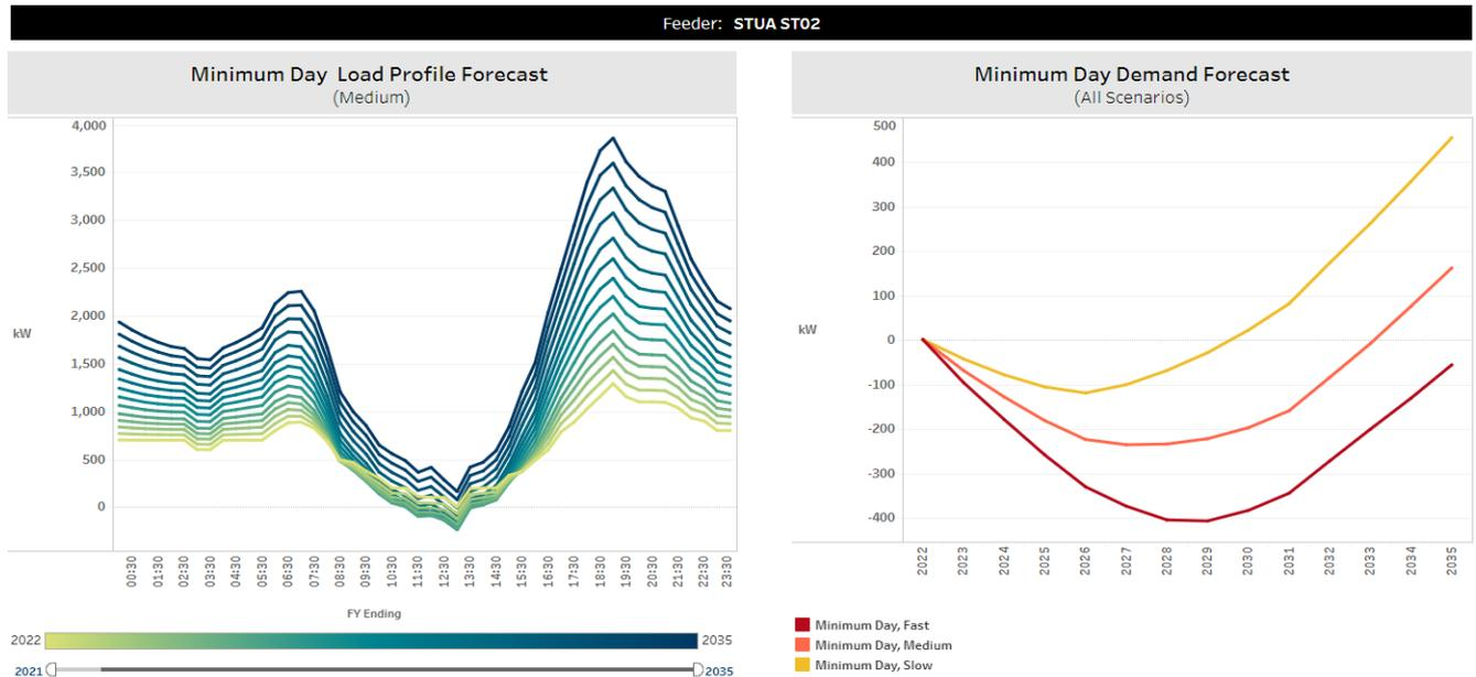
Figure 7 – ST-02 Feeder Minimum Demand Forecast
