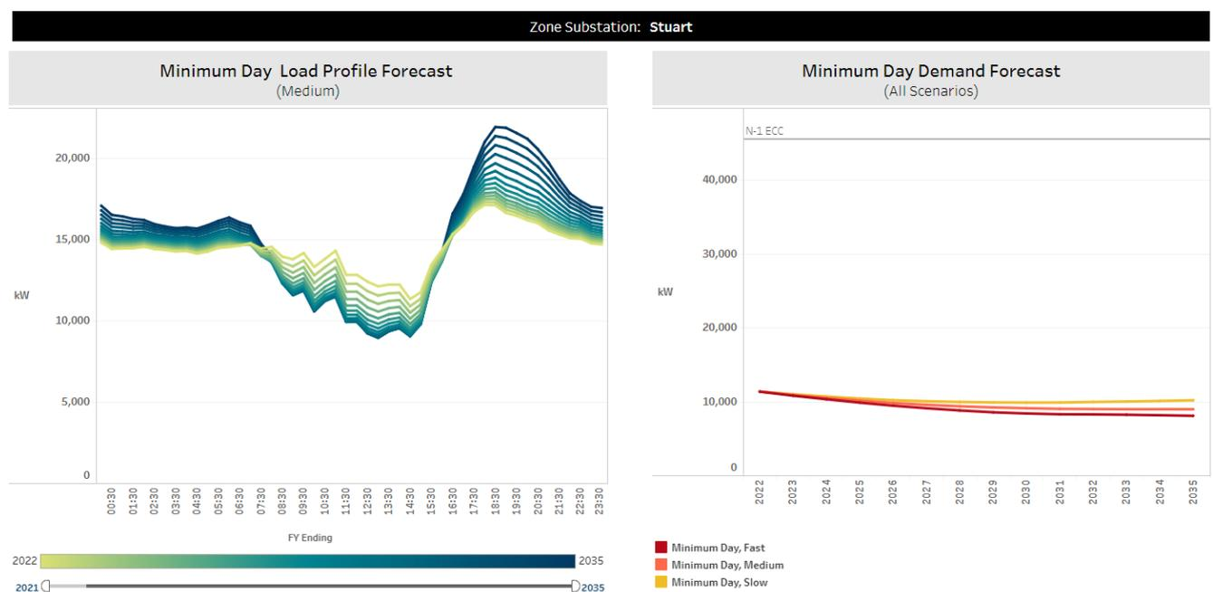
**Figure 6 – Stuart Substation Minimum Demand Forecast**
