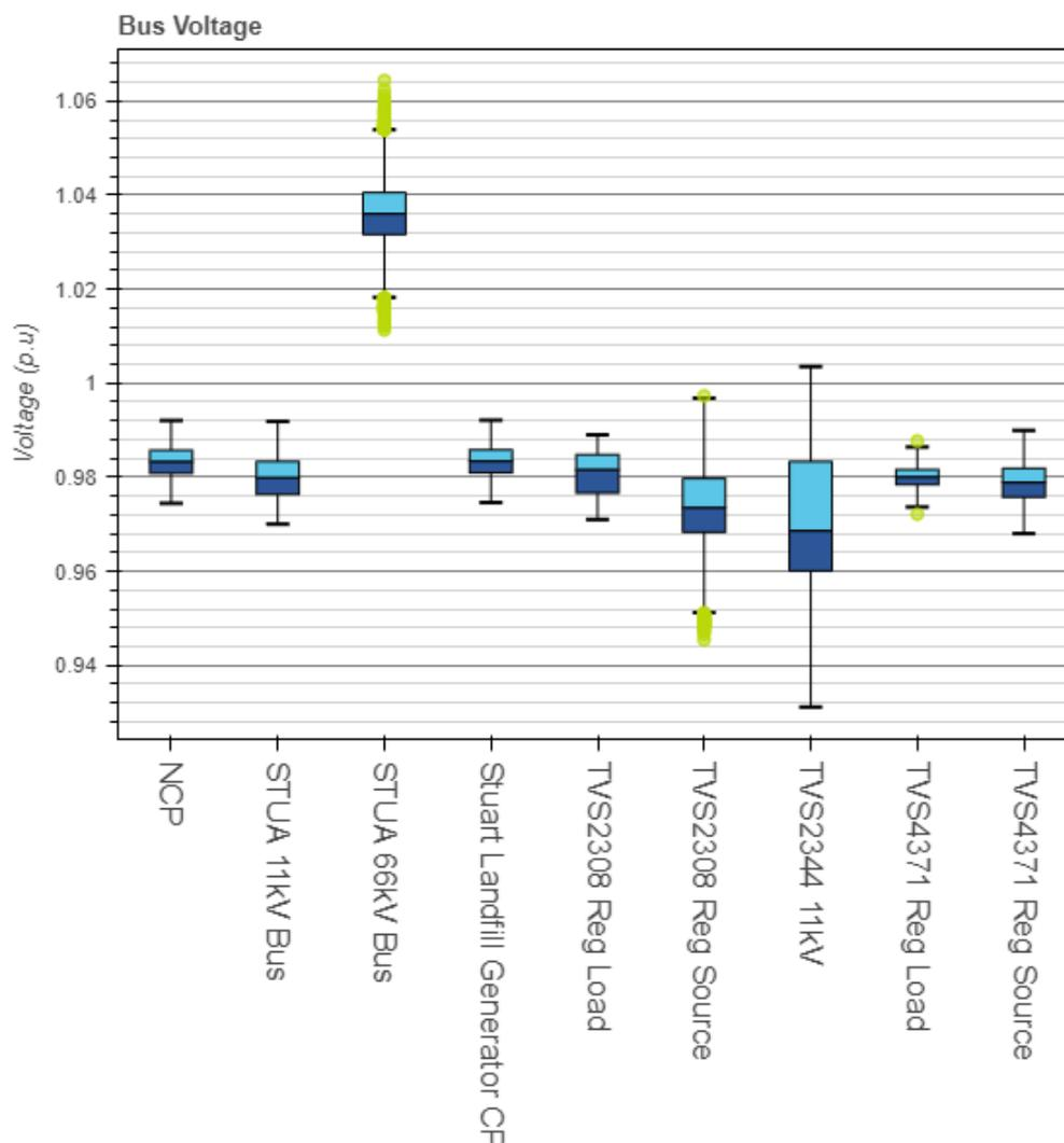
Figure 16 - Modelled voltages at key system nodes - Scenario 2 (Generator in Service)
