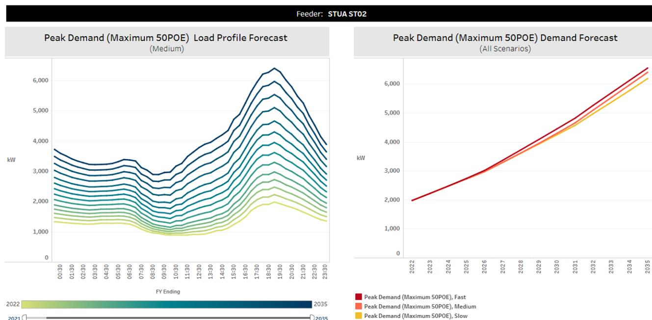
**Figure 9 – ST-02 Feeder Maximum Demand Forecast**
