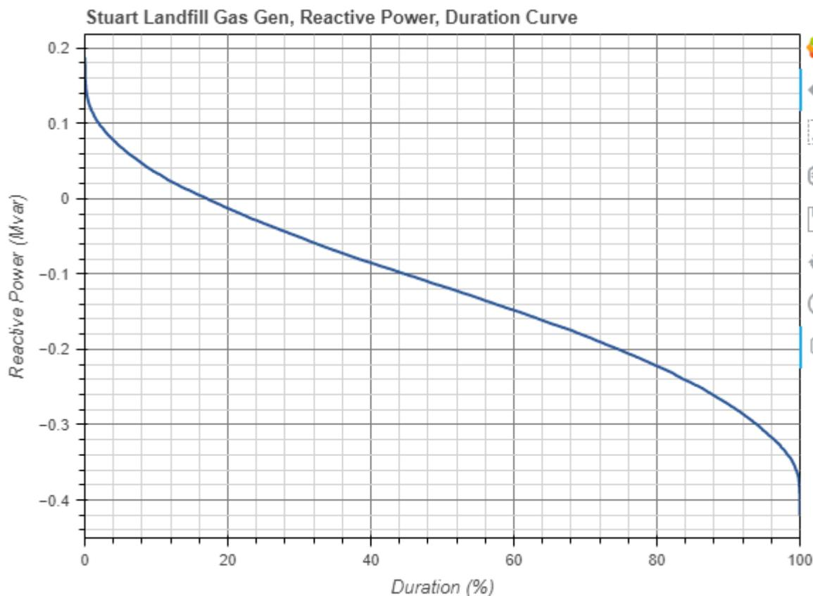
Figure 19 - Reactive Power Load Duration Curve
