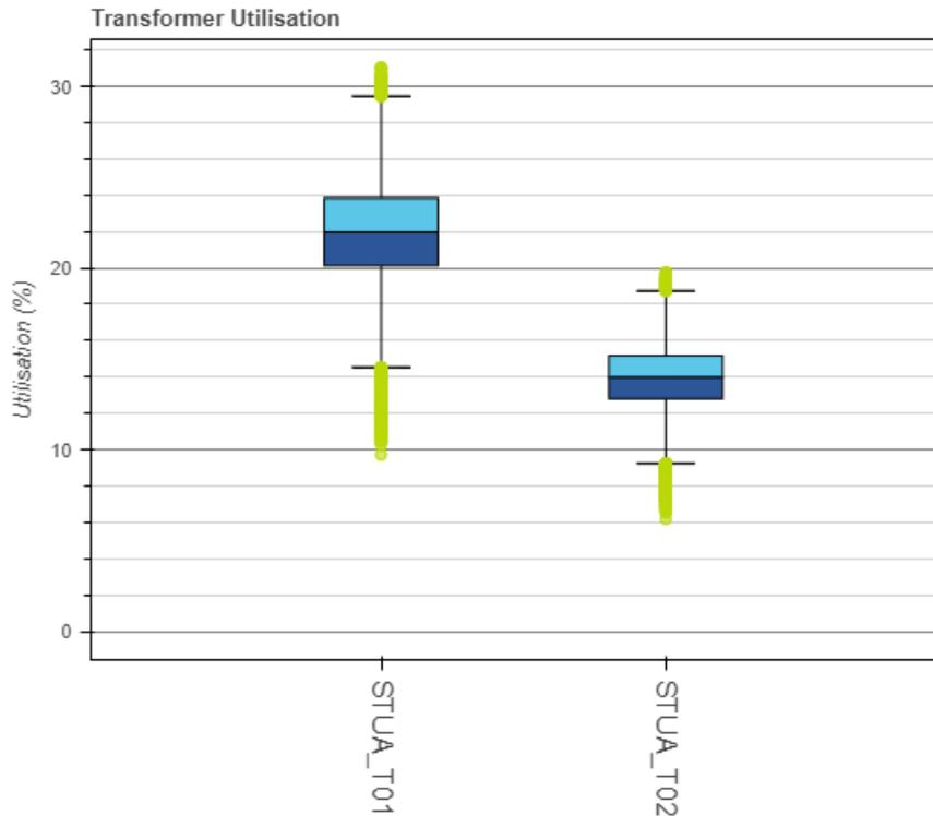
**Figure 13 - Existing Utilisation of Stuart 66/11kV (STUA) Substation Transformers**
