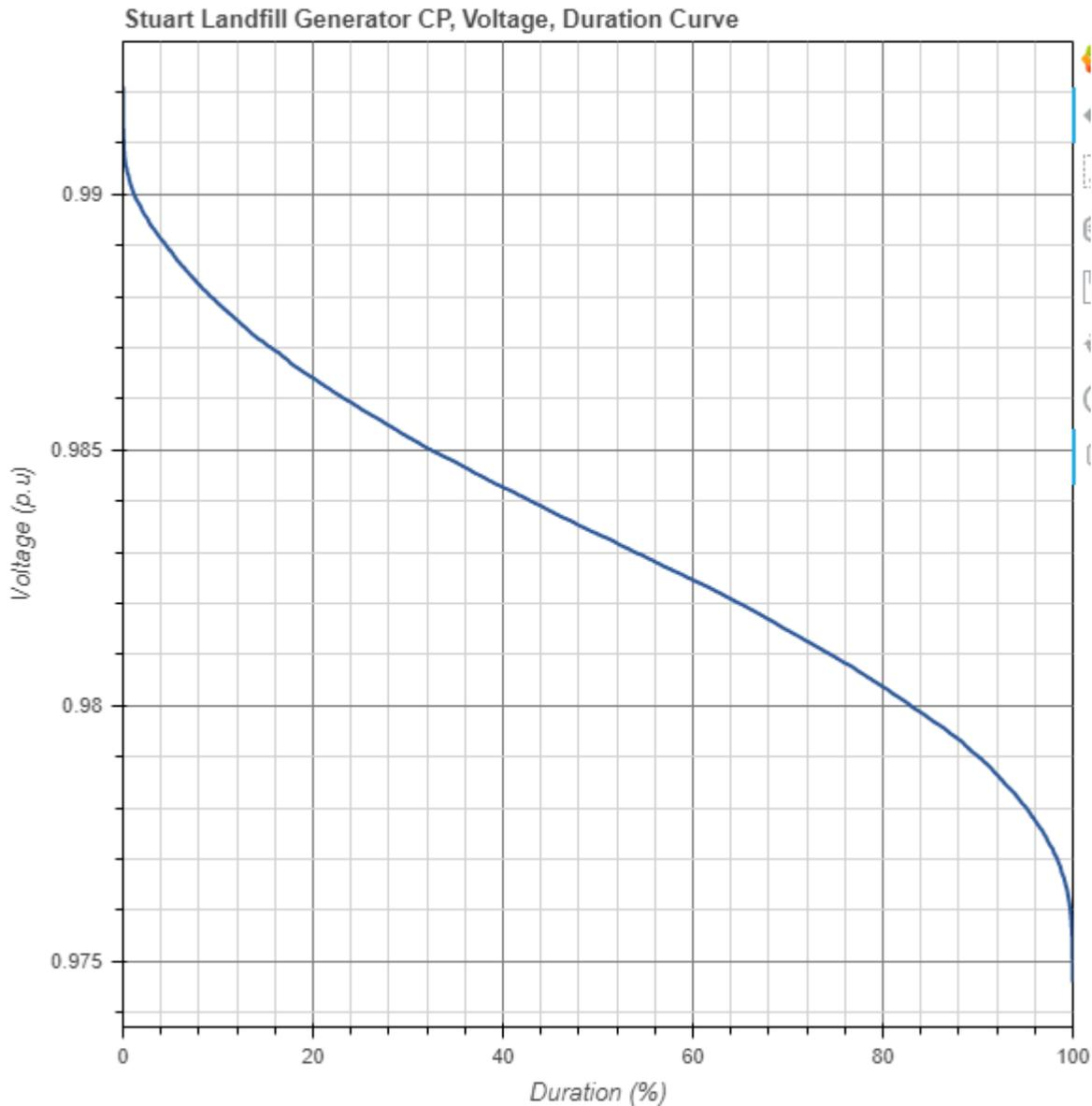
**Figure 17 - Connection Point Voltage Duration Curve - Scenario 2 (Generator in Service)**
