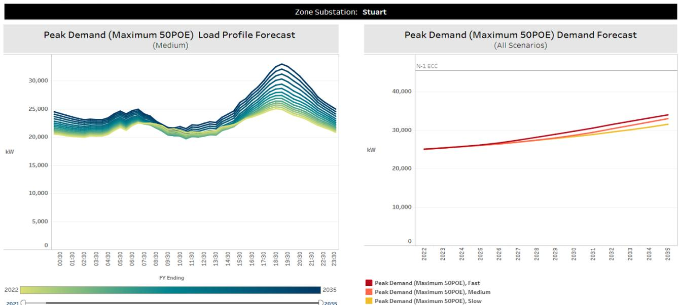
Figure 8 – Stuart Substation Maximum Demand Forecast
