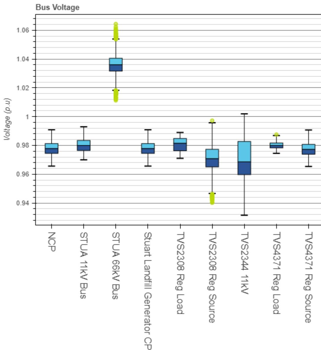
**Figure 10 - Modelled voltages at key system nodes - Scenario 1 (Base Case)**
