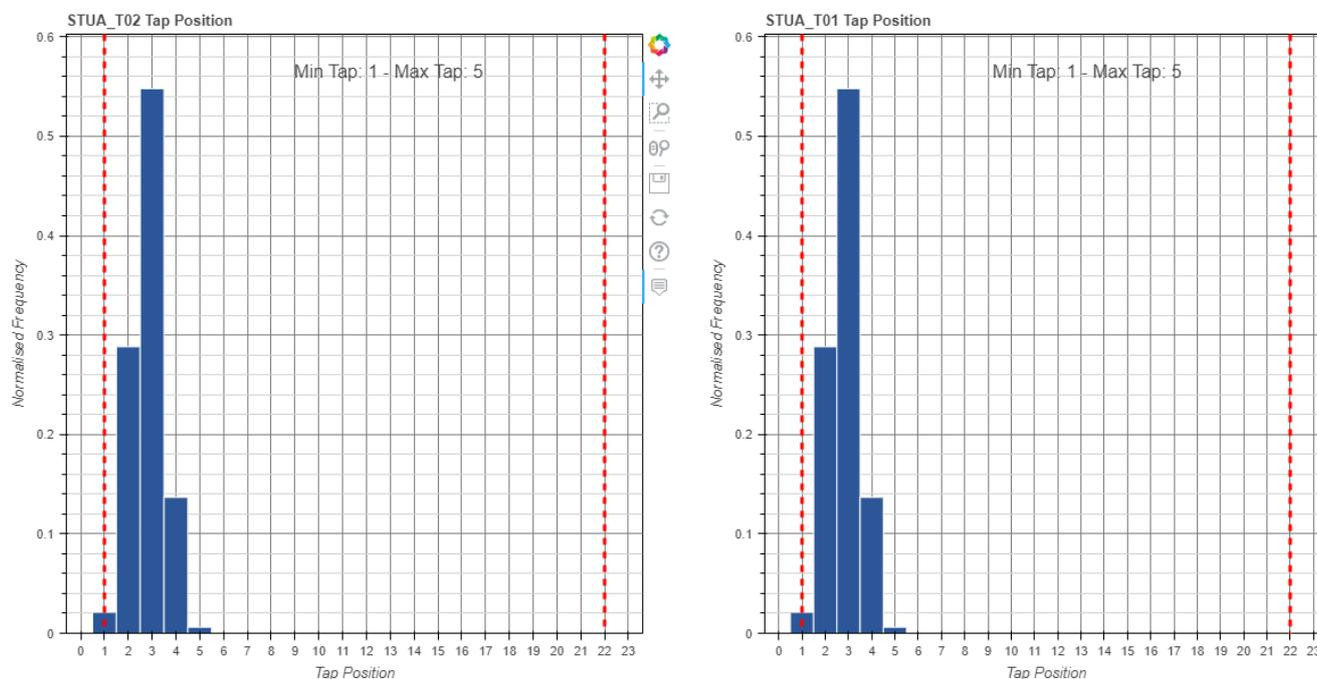
**Figure 23 - Anticipated Stuart 66/11kV (STUA) Substation Transformer Tap Position**
