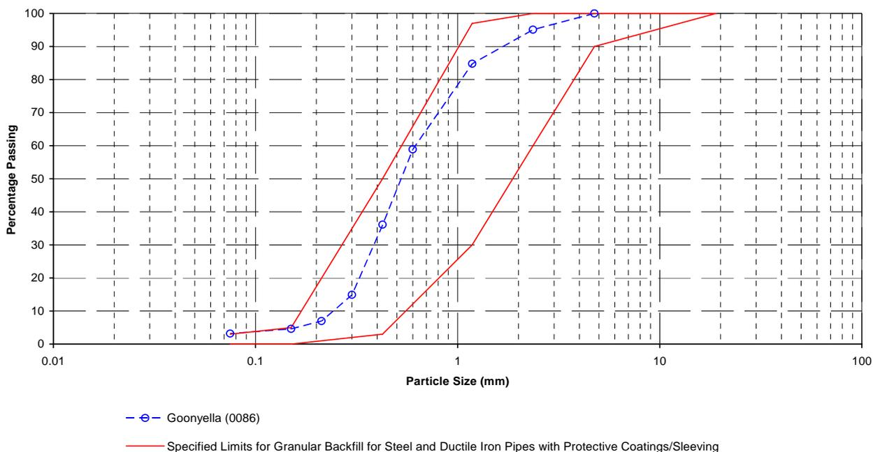
Figure 2: Isaac River Sand Grading Curve, Goonyella
