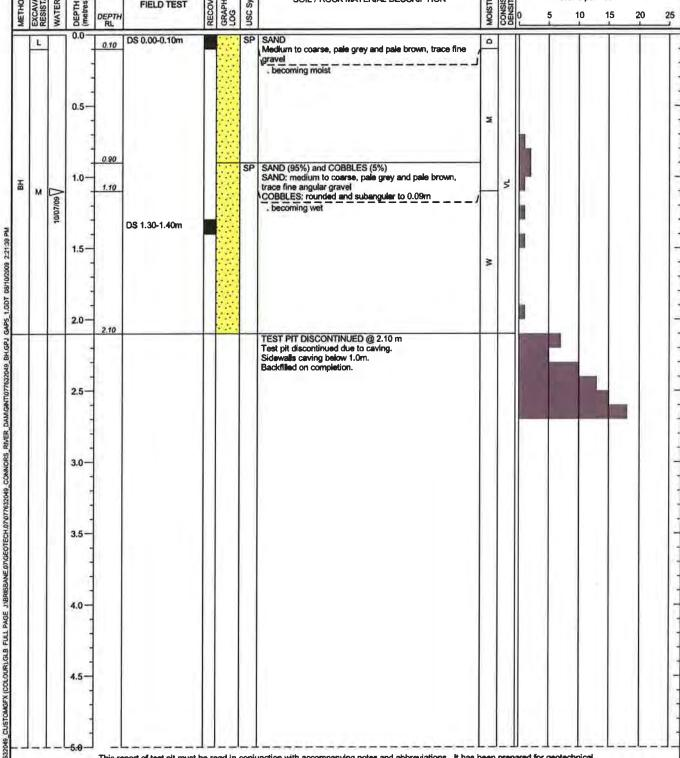
This report of test pit must be read in conjunction with accompanying notes and abbreviations. It has been prepared for geotechnical purposes only, without attempt to assess possible contamination. Any references to potential contamination are for information only and do not necessarily indicate the presence or absence of soil or groundwater contamination.
