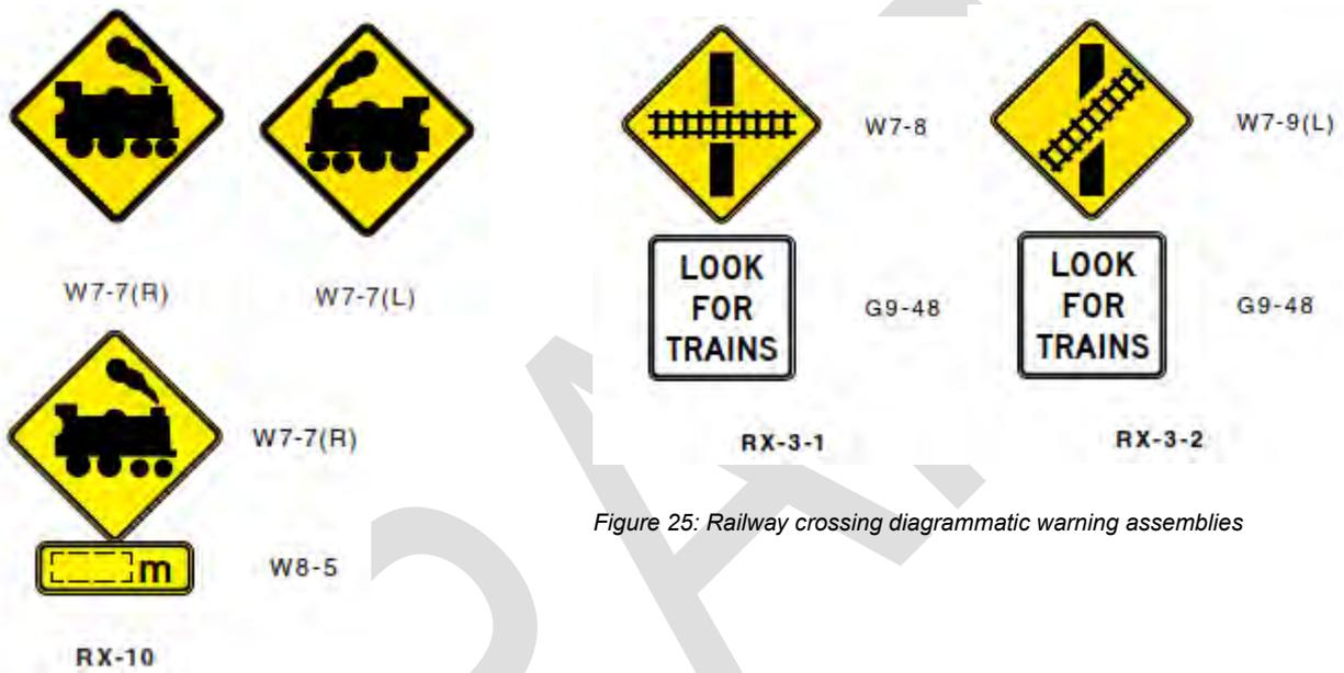
Figure 25: Railway crossing diagrammatic warning assemblies
