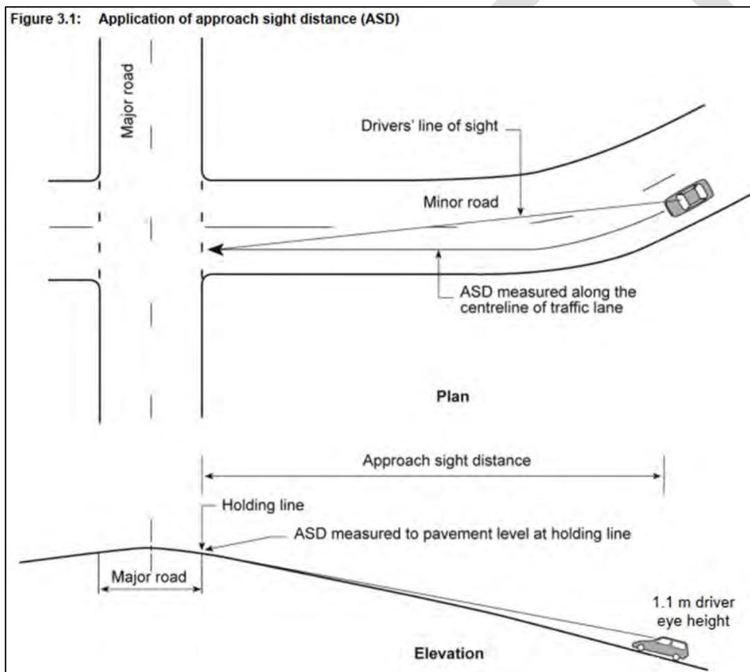
Figure 15: *Austrroads Guide to Road Design Part 4A: unsignalised and signalised intersections application of ASD*
