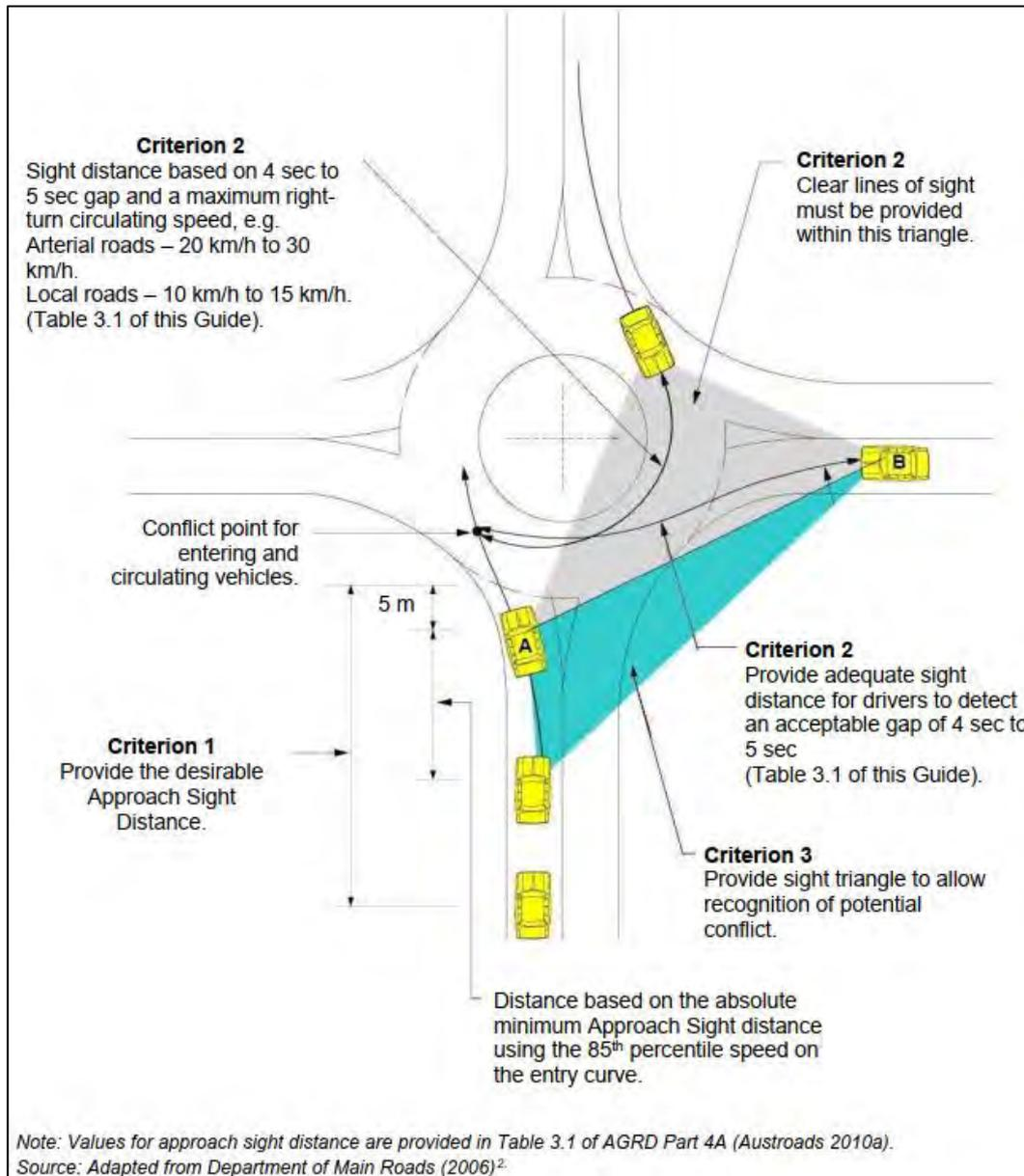
Figure 19: Austroads Guide to Road Design Part 4B: roundabouts sight distance criteria for roundabouts
