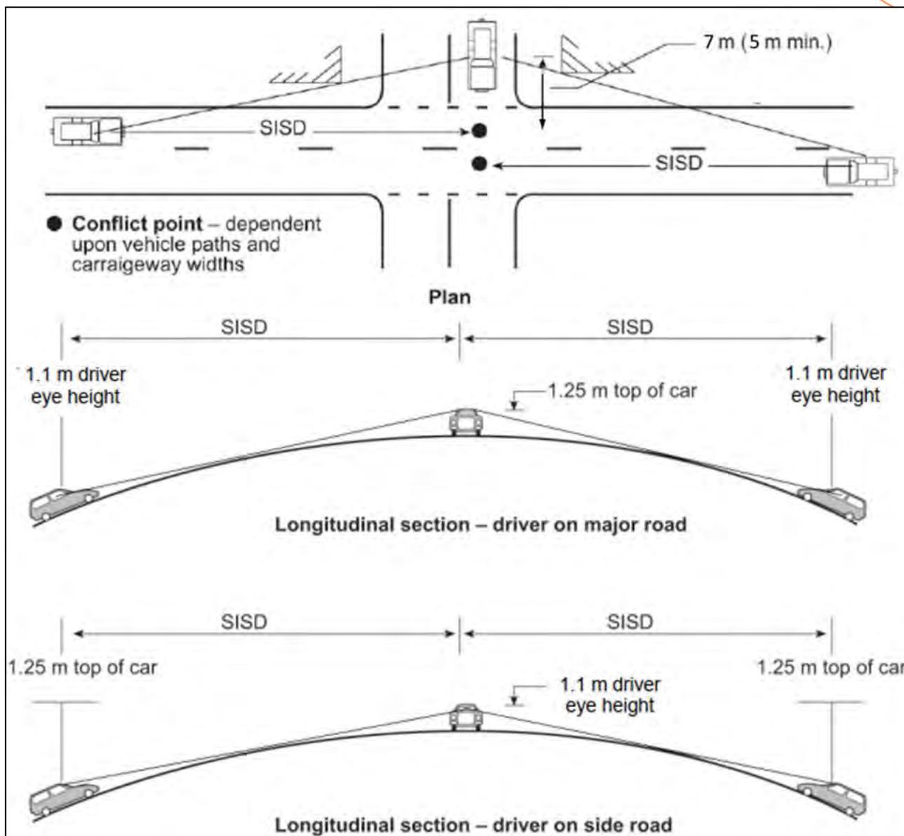
Figure 17: Supplement to AGRD Part 4A SISD
