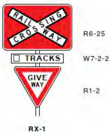
Figure 22: Railway crossing give-way assembly (RX-1)
