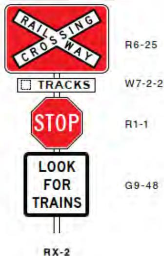
Figure 23: Railway crossing stop assembly (RX-2)
