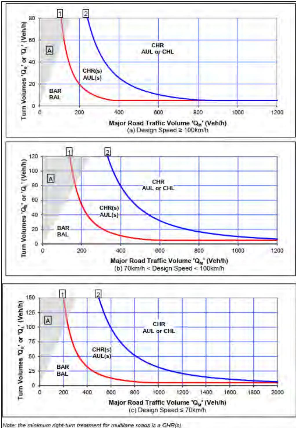
Figure 45: Warrants for turning treatments at unsignalised intersections (AGTM Part 6)
