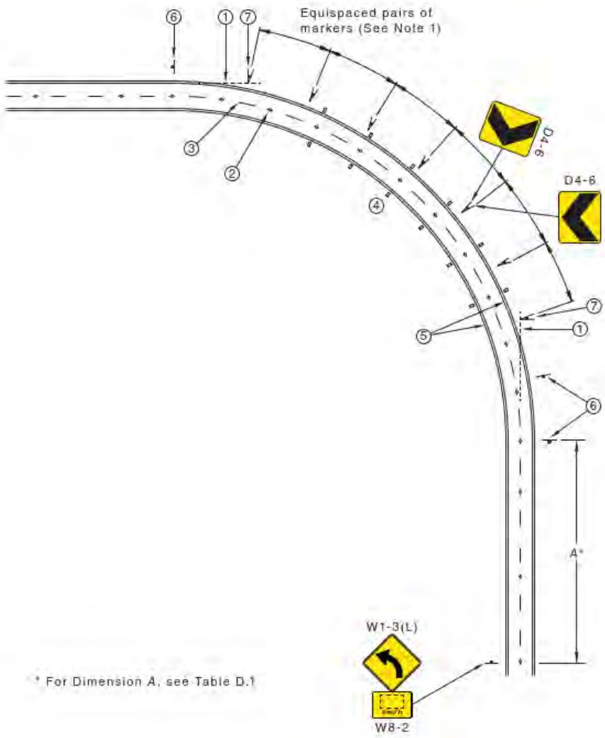
Figure 44: Example of curve warning signage (Source: AS 1742.2)
