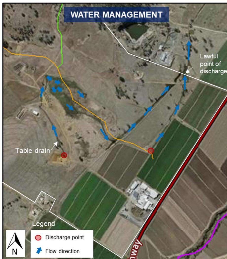
**Figure 2.** Processing water discharge points.
