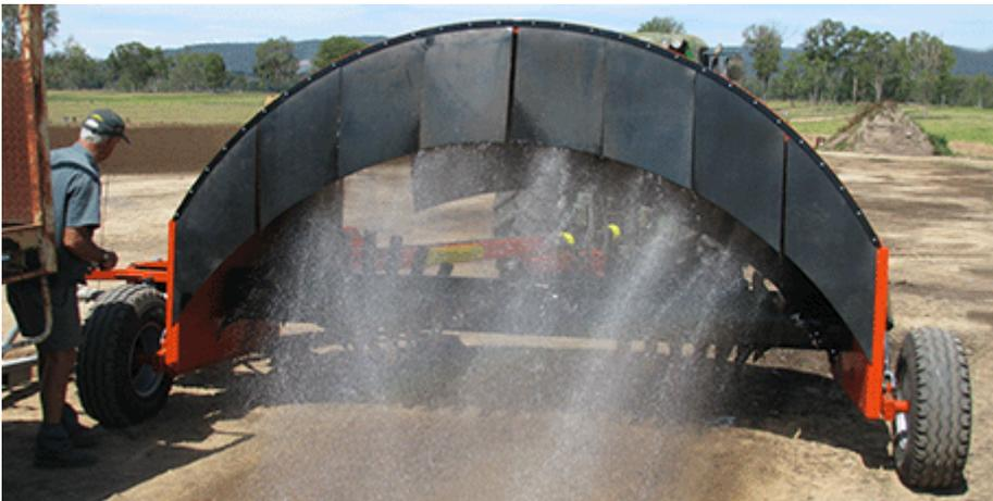
**Figure 1. Compost is wetted during turning to reduce dust**
