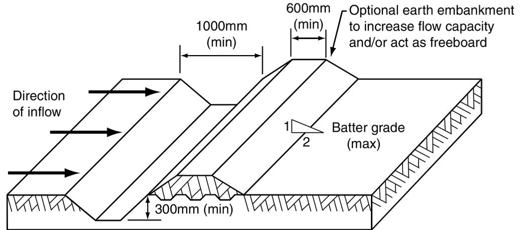
**Figure 1 - Typical profile of diversion channel with bank**
