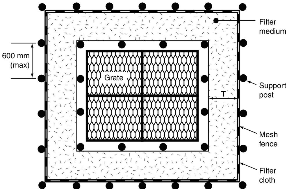
(c) Sediment weir drop inlet protection (plan view)
