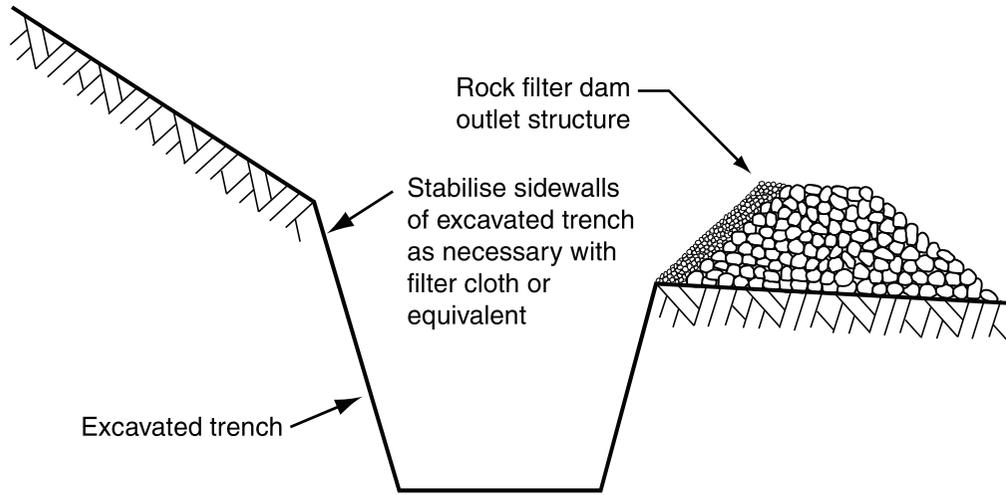
**(a) Sediment trench with rock filter dam outlet**
