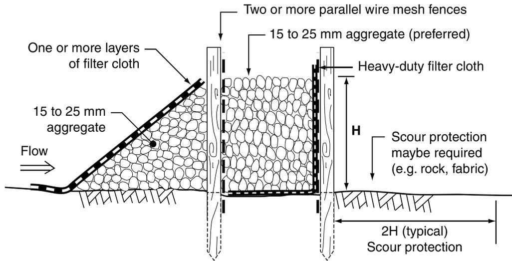
(a) Sediment weir with aggregate and geotextile filter
