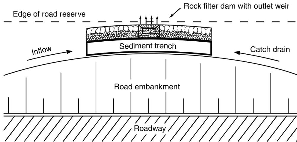
**(c) Typical layout of sediment trench at base of fill embankment**
