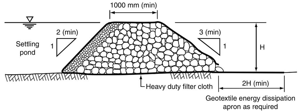
**(b) Rock filter dam outlet structure**
