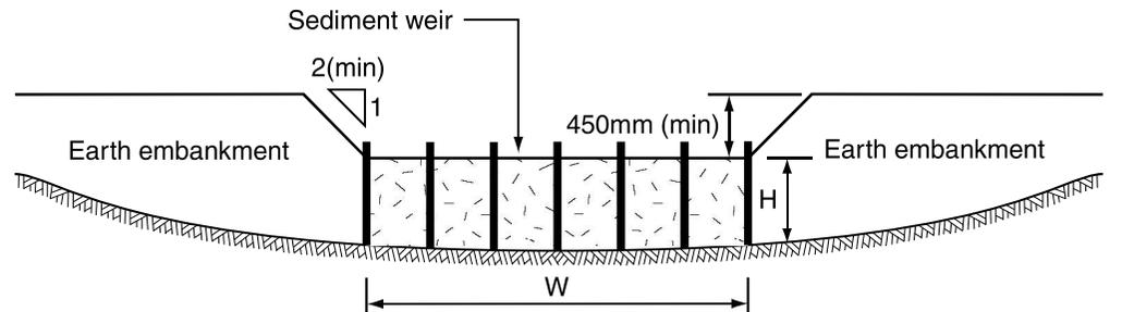
(d) Sediment weir with constructed earth abutments
