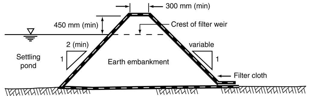
**(d) Typical cross-section of adjoining earth abutments (if required)**
