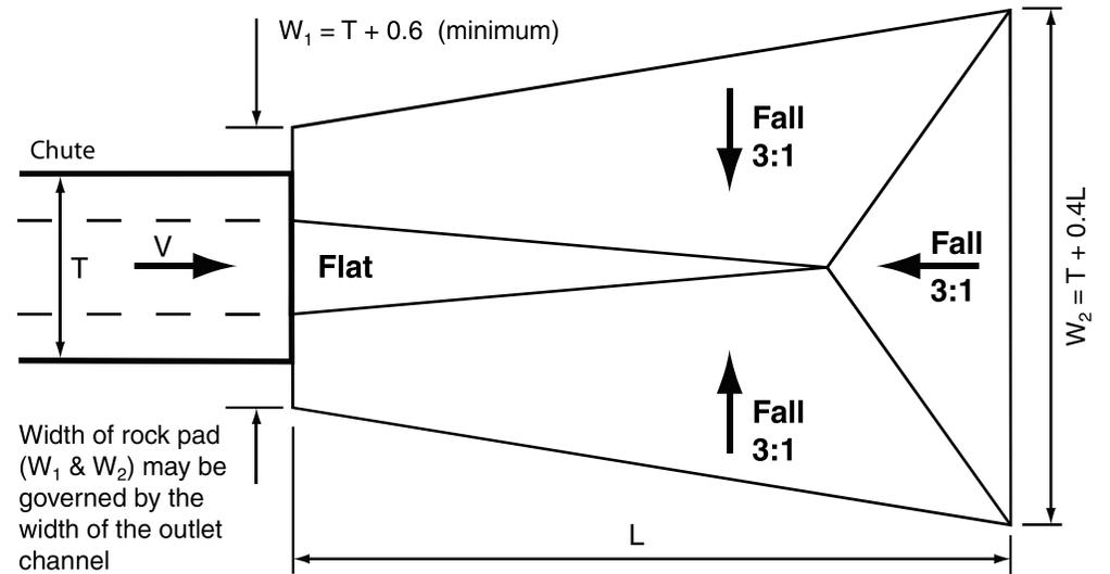
T = Maximum top width of flow at base of chute
