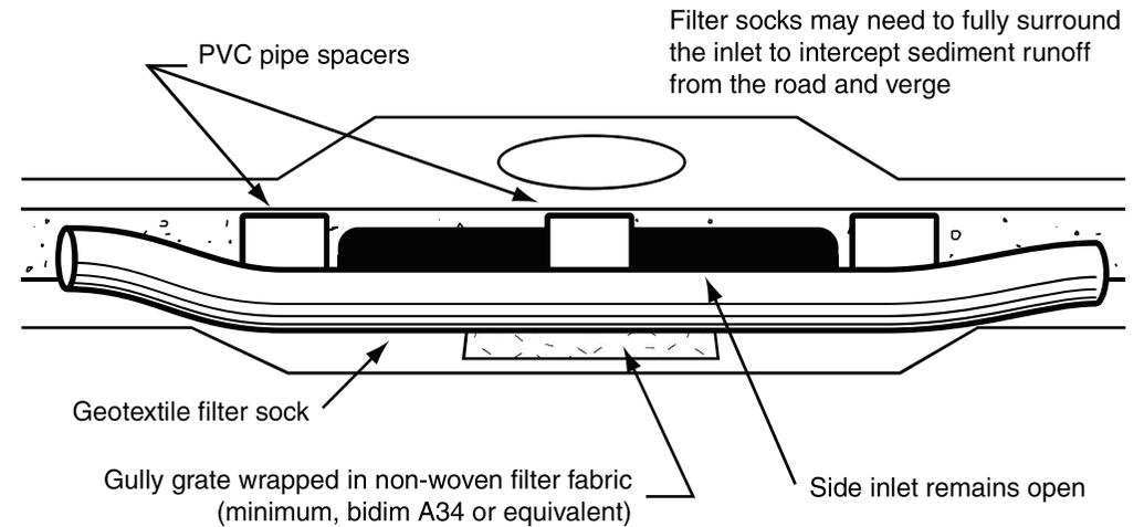
**(a) Filter sock sediment trap on a sag inlet**
