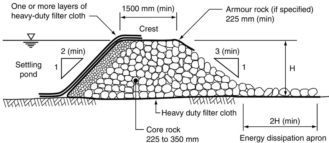
**(a) Rock filter dam with aggregate filter
