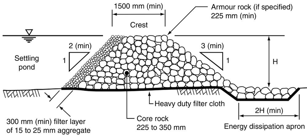
**(a) Rock filter dam with aggregate filter**
