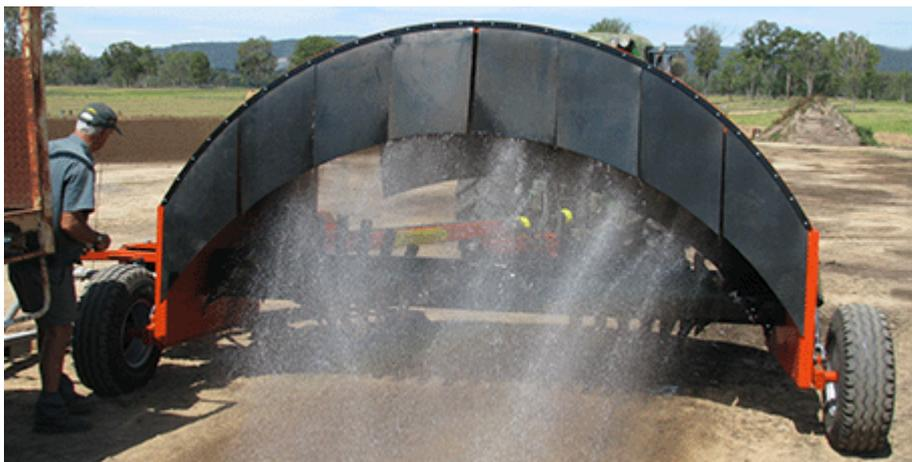
**Figure 56. Compost is wetted while being turned to reduce dust**
