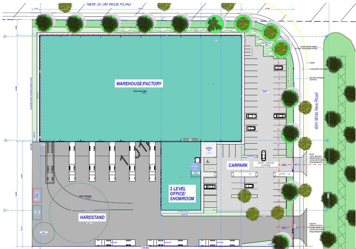
Figure 32. Site Plan of Warehouse, Showroom and Ancillary Office
