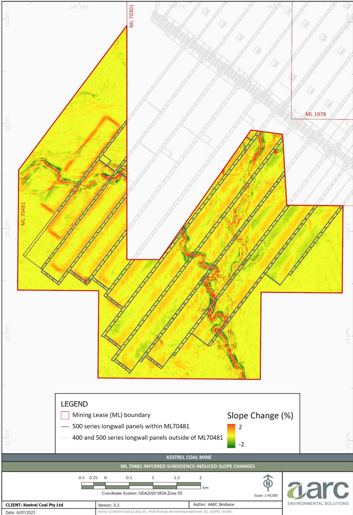
Figure 10: Inferred subsidence-induced slope changes between +2% and -2%
