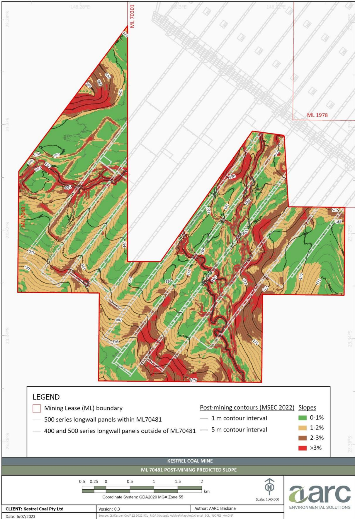
Figure 9: Inferred slope gradient classes post-mining (MSEC [2022] predicted subsidence DEM)
