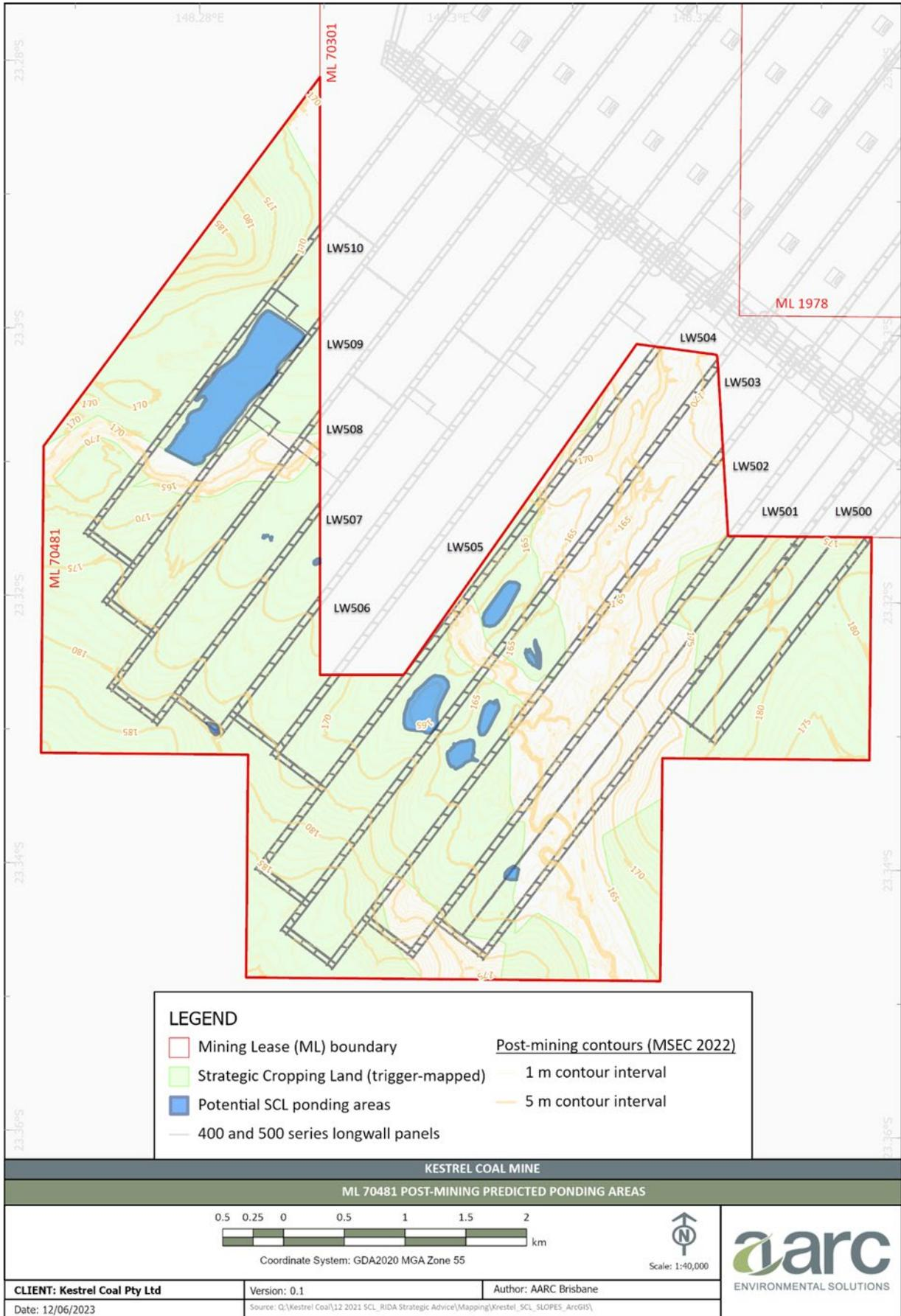
Figure 11: Inferred ponding subsequent to subsidence (revised mine plan incl. LW510)
