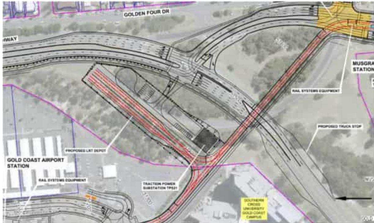
Figure 33 Bilonga LRT satellite depot and stabling yard
