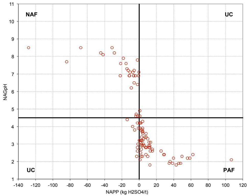
Figure 9: ARD classification plot showing NAGpH versus NAPP for fresh Permian samples, with ARD classification domains indicated.
