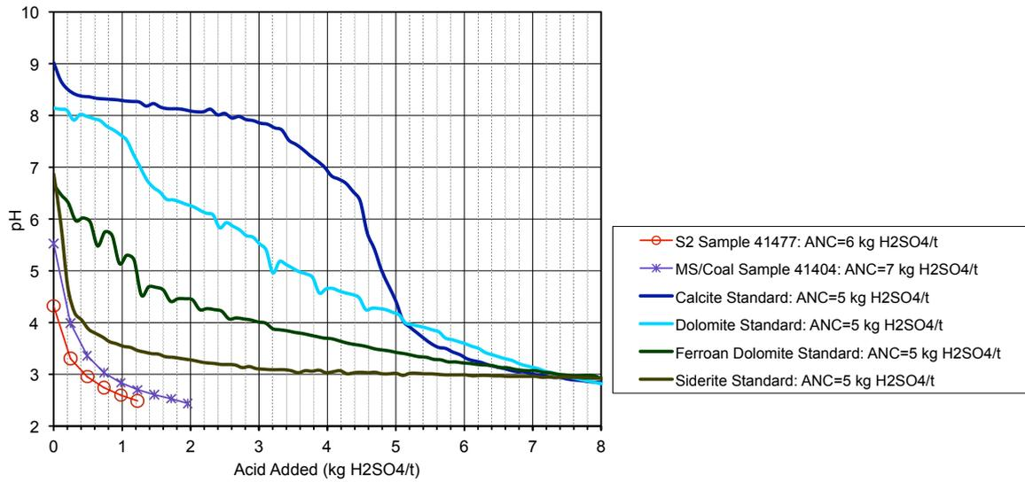
Figure 10: ABCC profile for samples with an ANC value close to 5 kg H<sub>2</sub>SO<sub>4</sub>/t. Carbonate standard curves are included for reference.
