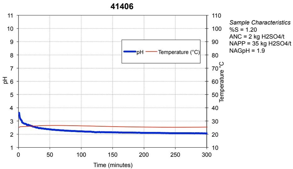
Figure 20: Kinetic NAG graph for sample 41406.
