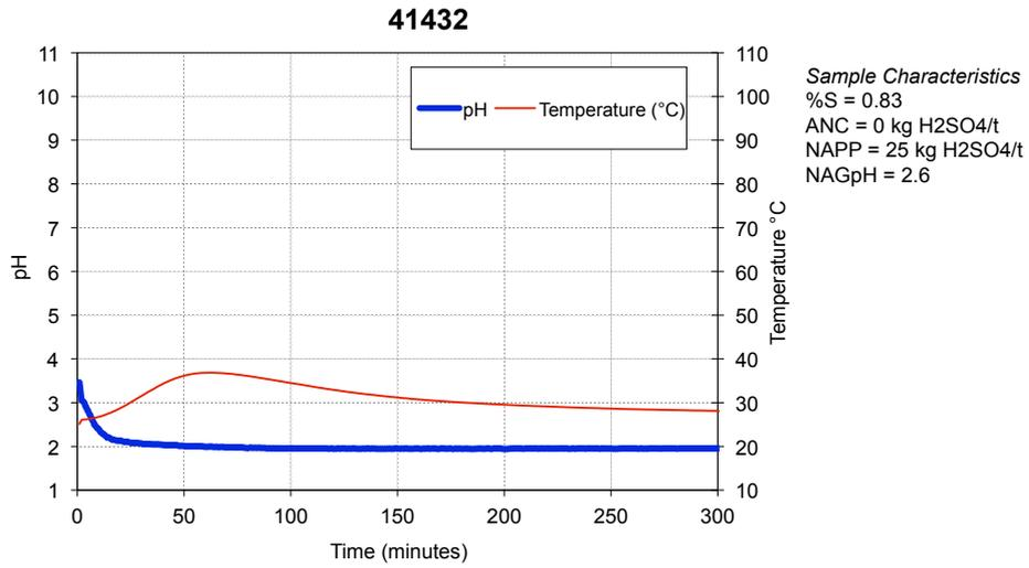
Figure 18: Kinetic NAG graph for sample 41432.
