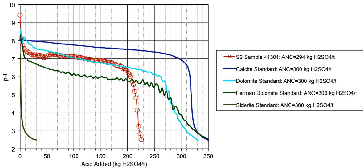
Figure 17: ABCC profile for sample 41301 with an ANC value close to 300 kg H<sub>2</sub>SO<sub>4</sub>/t. Carbonate standard curves are included for reference.
