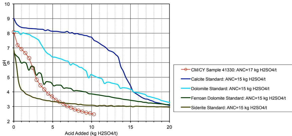
Figure 12: ABCC profile for sample 41330 with an ANC value close to 15 kg H<sub>2</sub>SO<sub>4</sub>/t. Carbonate standard curves are included for reference.
