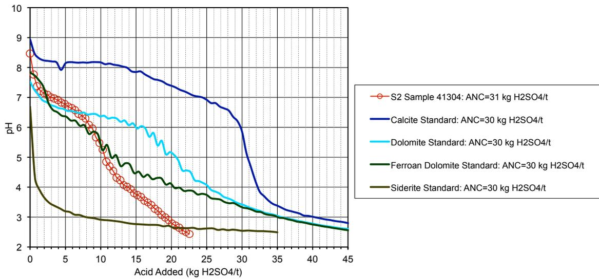
Figure 14: ABCC profile for sample 41304 with an ANC value close to 30 kg H<sub>2</sub>SO<sub>4</sub>/t. Carbonate standard curves are included for reference.
