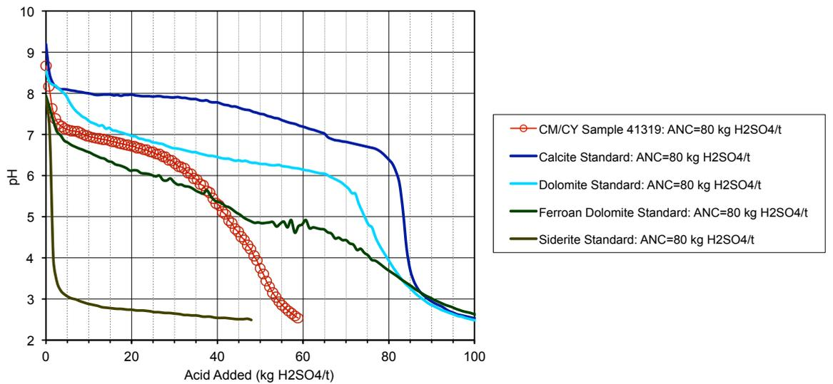
Figure 15: ABCC profile for sample 41319 with an ANC value of 80 kg H<sub>2</sub>SO<sub>4</sub>/t. Carbonate standard curves are included for reference.
