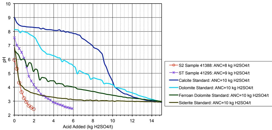
Figure 11: ABCC profile for samples with an ANC value close to 10 kg H<sub>2</sub>SO<sub>4</sub>/t. Carbonate standard curves are included for reference.
