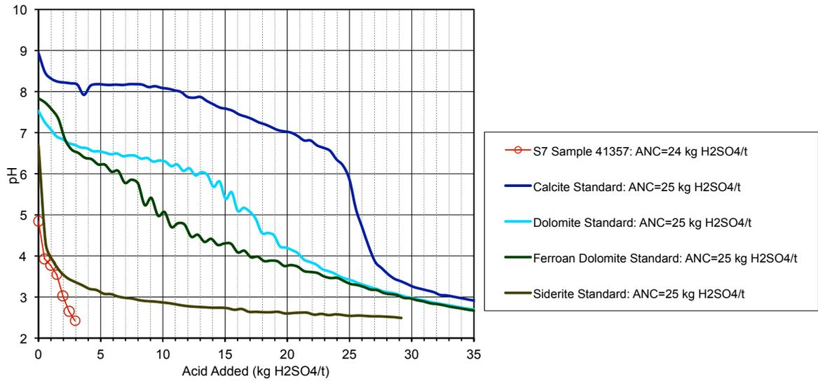
Figure 13: ABCC profile for sample 41357 with an ANC value close to 25 kg H<sub>2</sub>SO<sub>4</sub>/t. Carbonate standard curves are included for reference.
