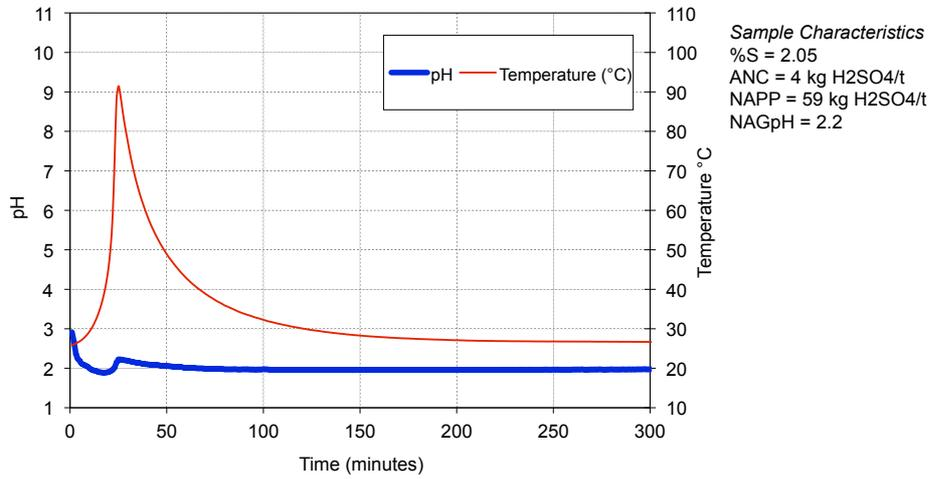
Figure 22: Kinetic NAG graph for sample 41349.
