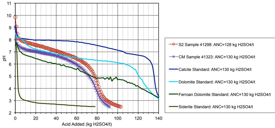
Figure 16: ABCC profile for samples with an ANC value close to 130 kg H<sub>2</sub>SO<sub>4</sub>/t. Carbonate standard curves are included for reference.
