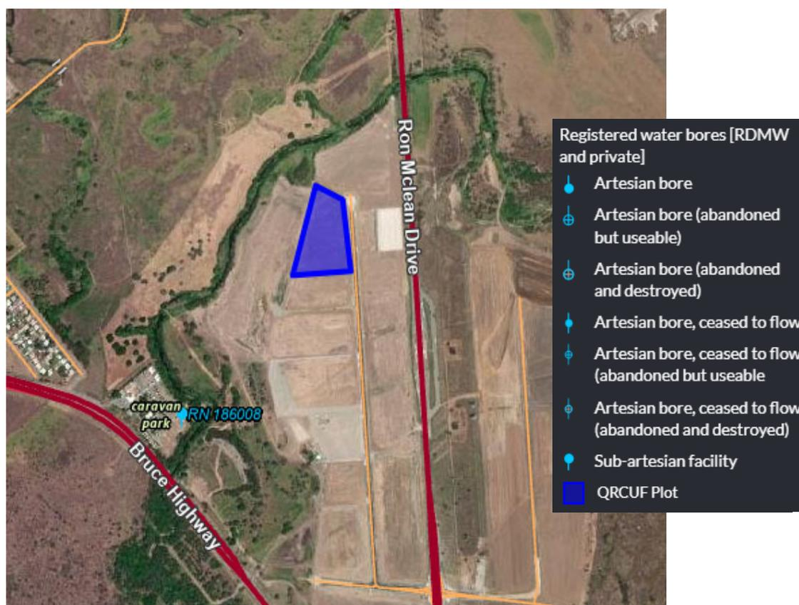
Figure 3-10: Registered groundwater bores surrounding QRCUF.
