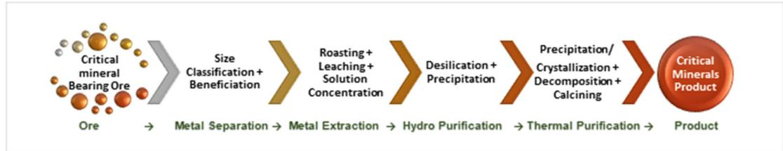
Figure 2-2: Basic mineral recovery process
