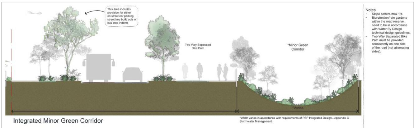
Figure 1: Cross sections for minor green corridor<sup>6</sup>
