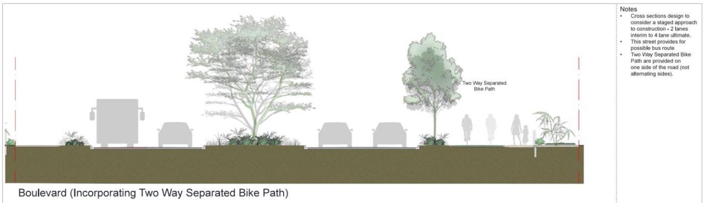
**Figure 2: Cross sections for two way separated bike path<sup>7</sup>**
