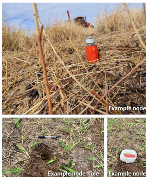
**Plate 3.3** Example of Seismic Receivers Node and In-ground Placement
