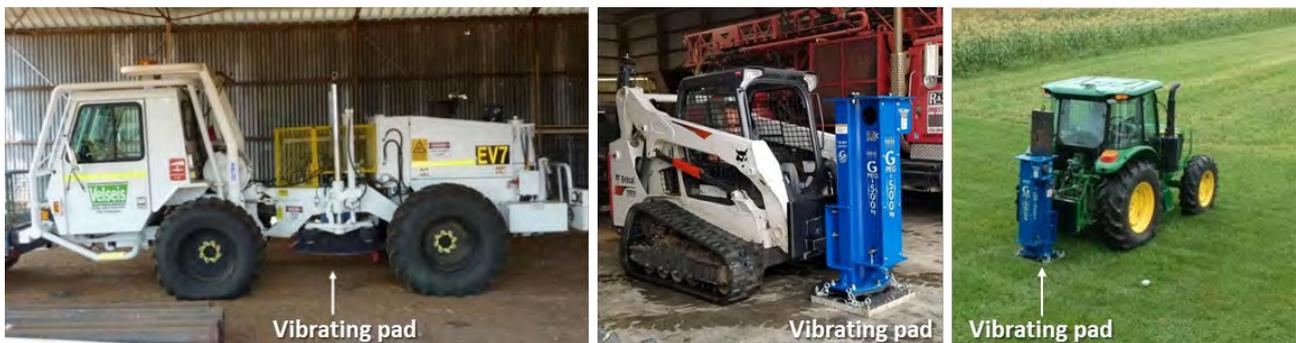
**Plate 3.4**      **Examples of Energy Source Vehicles with Vibrating Pad (EnviroVibe, Bobcat, Tractor)**
