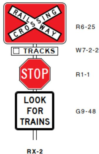
Figure 23: Railway crossing stop assembly (RX-2)
