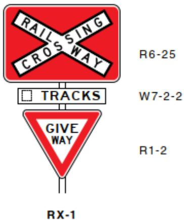
Figure 22: Railway crossing give-way assembly (RX-1)
