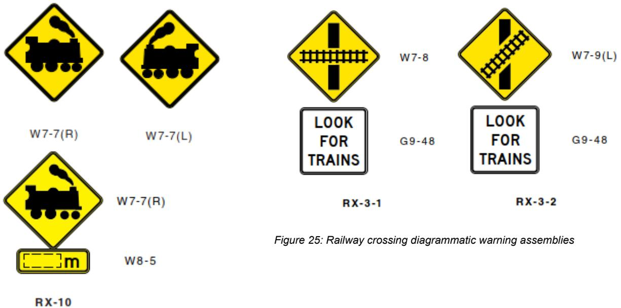
Figure 25: Railway crossing diagrammatic warning assemblies
