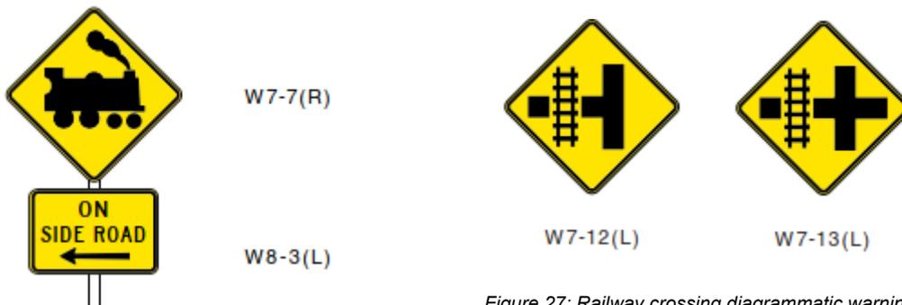
Figure 27: Railway crossing diagrammatic warning assemblies – on side road
