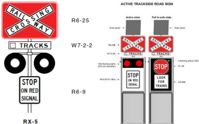
Figure 29: Railway crossing flashing signal assembly
