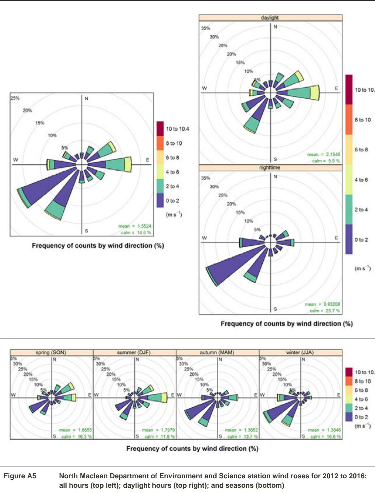
**Figure A5** North Maclean Department of Environment and Science station wind roses for 2012 to 2016: all hours (top left); daylight hours (top right); and seasons (bottom)
