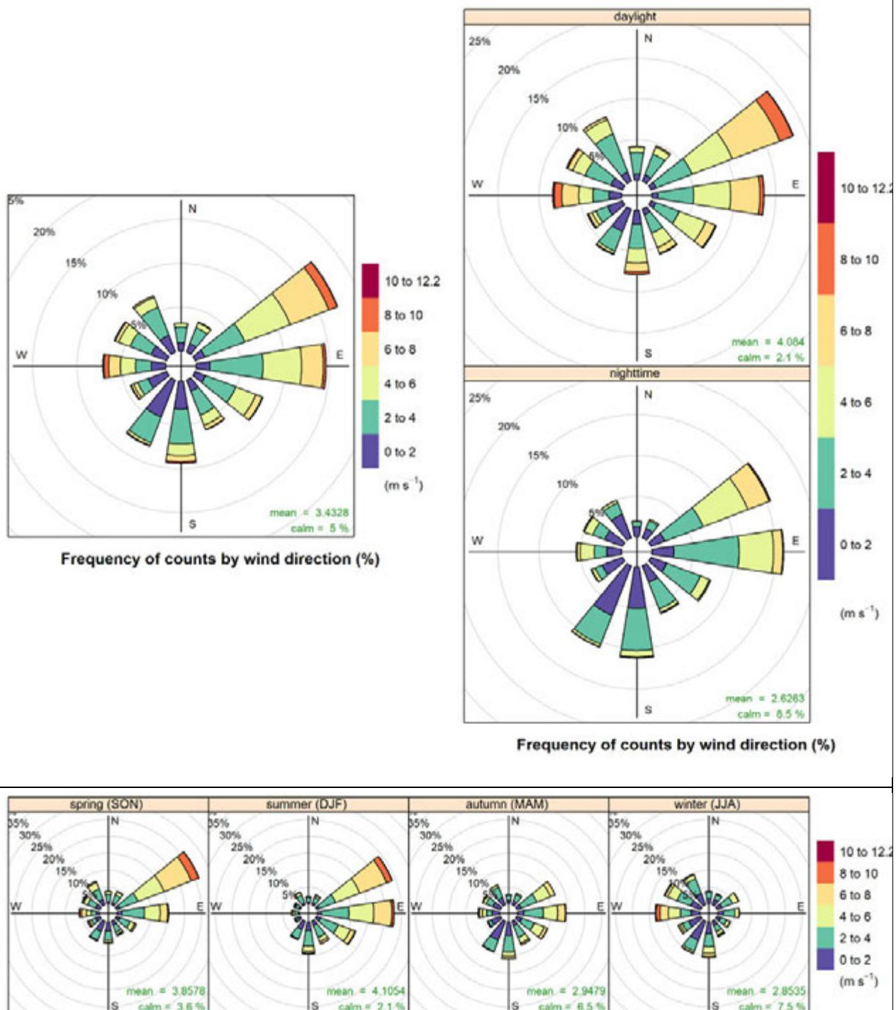
**Figure A2**      Amberley AMO Bureau of Meteorology station wind roses for 2012 to 2016: all hours (top left); daylight hours (top right); and seasons (bottom)
