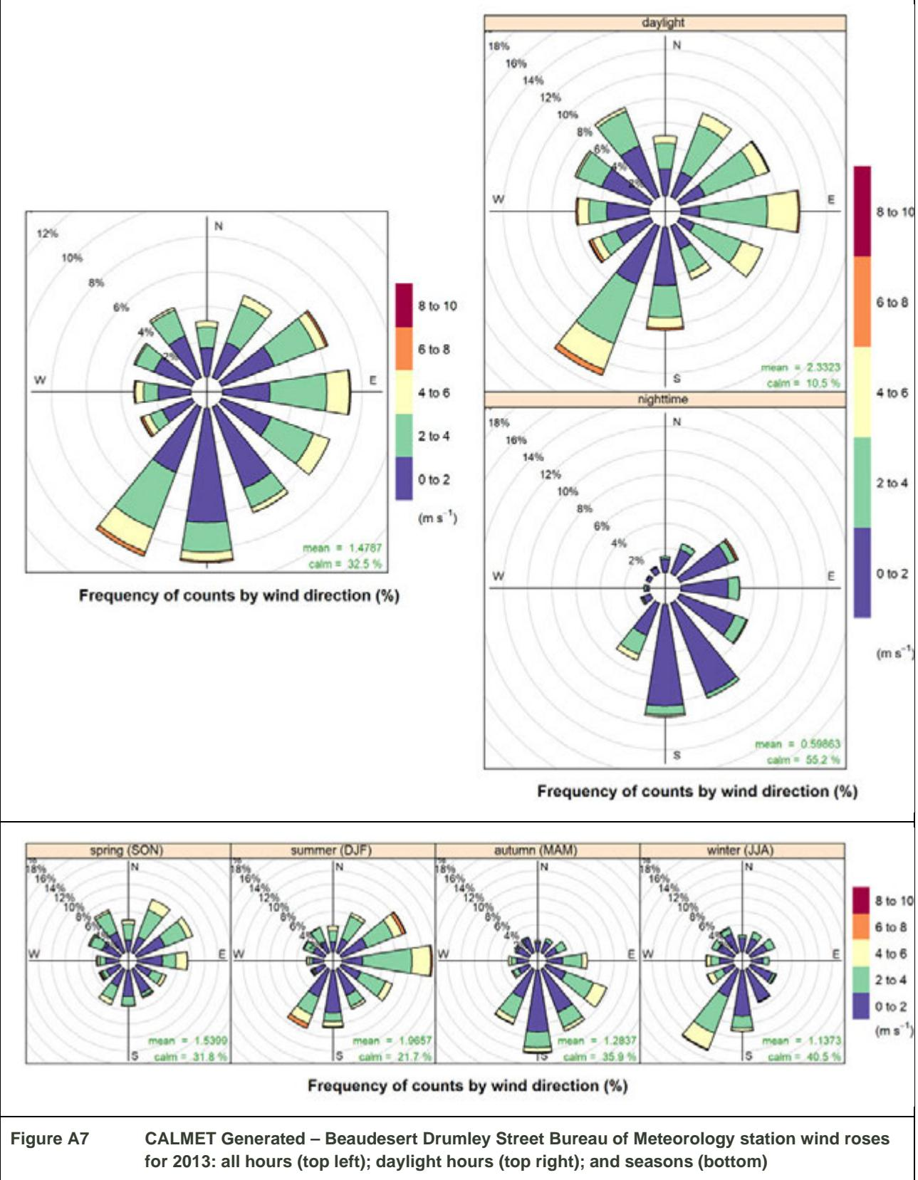
**Figure A7** CALMET Generated – Beaudesert Drumley Street Bureau of Meteorology station wind roses for 2013: all hours (top left); daylight hours (top right); and seasons (bottom)
