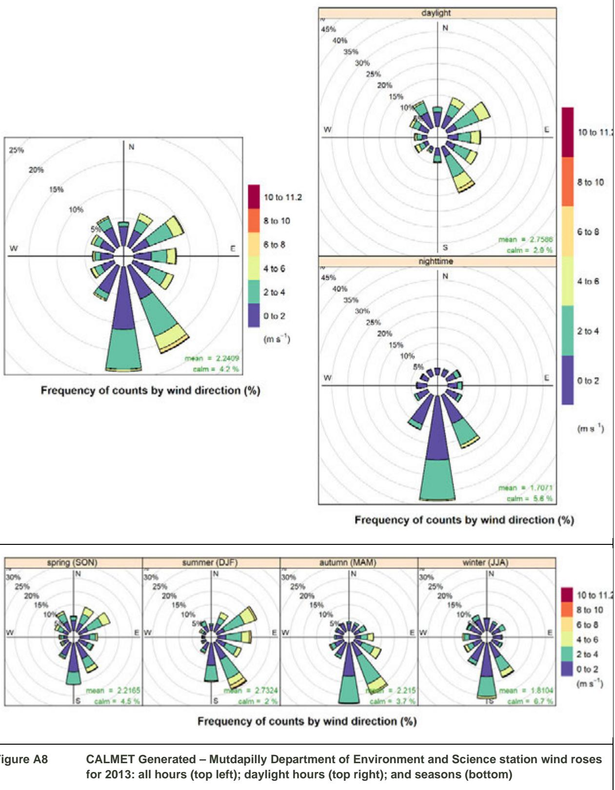
**Figure A8** CALMET Generated – Mutdapilly Department of Environment and Science station wind roses for 2013: all hours (top left); daylight hours (top right); and seasons (bottom)
