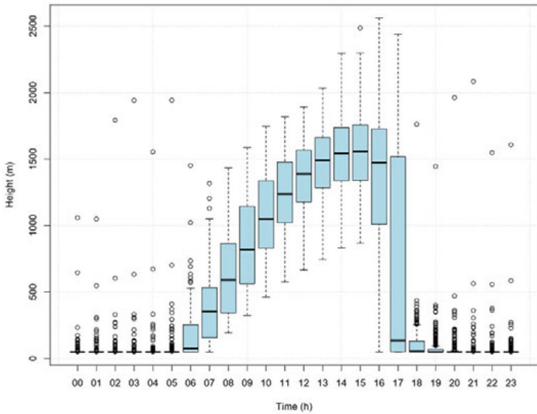
**Figure A13** Mixing height statistics by hour of day for Beaudesert Drumley Street Bureau of Meteorology site (CALMET Generated)
