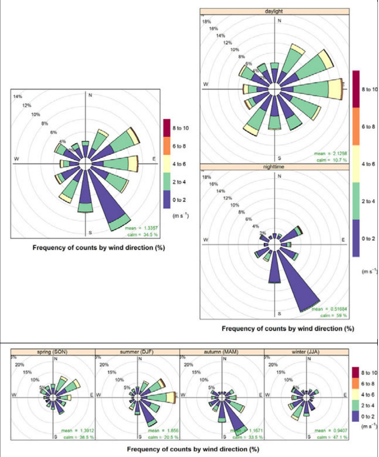
**Figure A10** CALMET Generated – West Portal Teviot Range Tunnel wind roses for 2013: all hours (top left); daylight hours (top right); and seasons (bottom)
