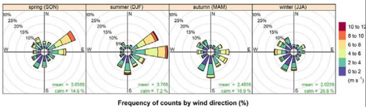
**Figure A6 CALMET Generated – Amberley AMO Bureau of Meteorology station wind roses for 2013: all hours (top left); daylight hours (top right); and seasons (bottom)**
