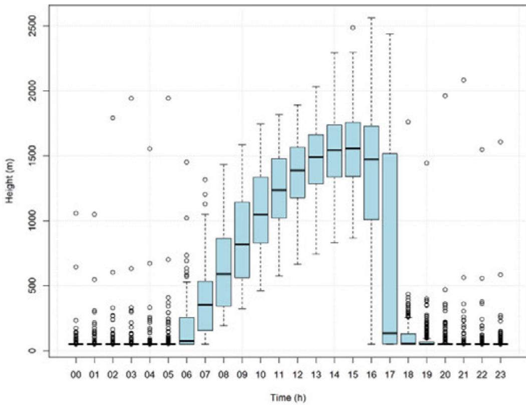
**Figure A12** Mixing height statistics by hour of day for Mutdapilly Department of Environment and Science site (CALMET Generated)
