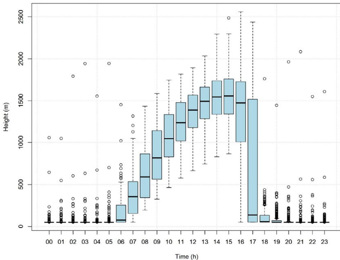
FIGURE 12.8: MIXING HEIGHT STATISTICS BY HOUR OF DAY FOR MUTDAPILLY DEPARTMENT OF ENVIRONMENT AND SCIENCE STATION (CALMET GENERATED)
