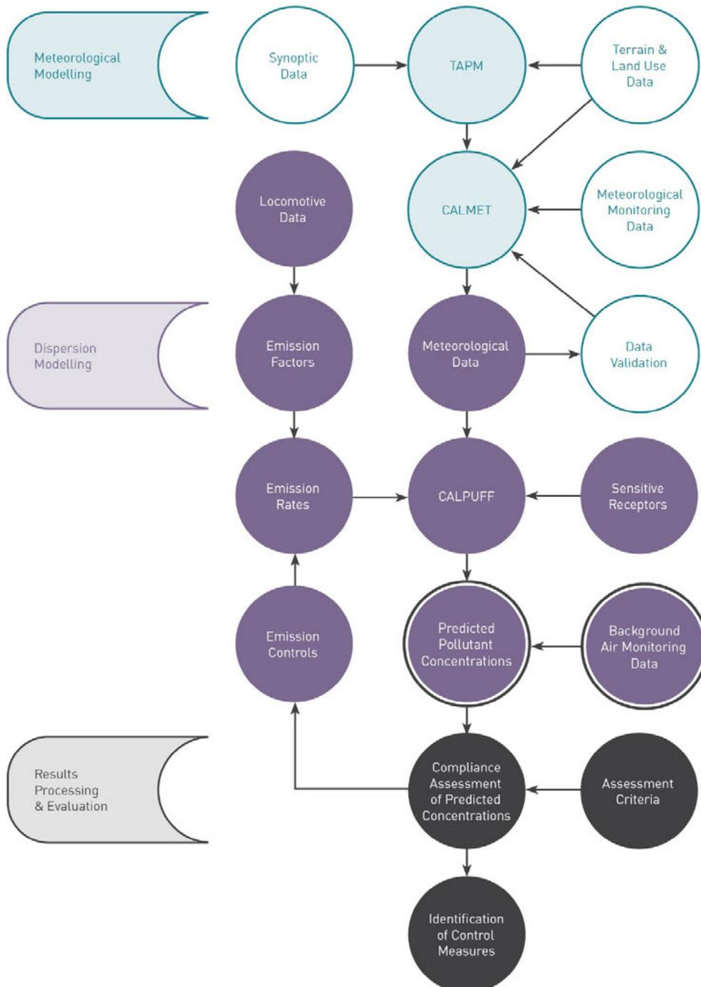
FIGURE 12.2: DIAGRAMMATIC REPRESENTATION OF THE CALPUFF MODELLING METHODOLOGY
