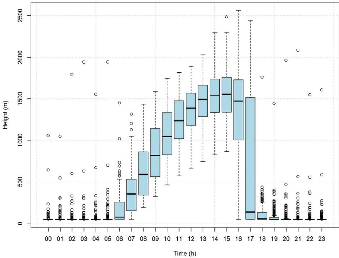
FIGURE 12.10: MIXING HEIGHT STATISTICS BY HOUR OF DAY FOR TEVIOT RANGE TUNNEL WESTERN PORTAL (CALMET GENERATED)
