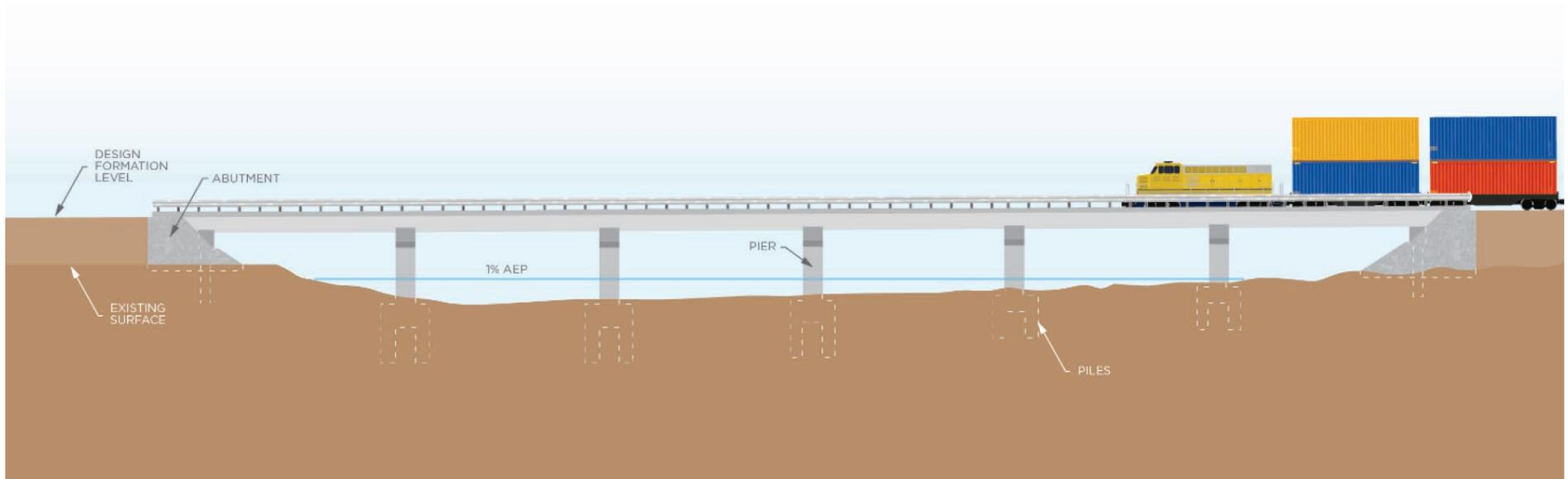
FIGURE 6.10: TYPICAL SECTION OF RAIL OVER WATERCOURSE BRIDGE STRUCTURE
