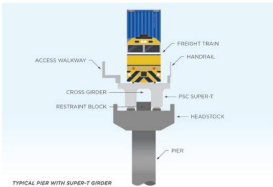
**FIGURE 6.8: TYPICAL PIER WITH PRE-STRESSED CONCRETE SUPER-T GIRDER**
