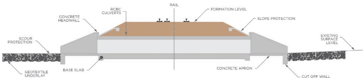
FIGURE 6.13: TYPICAL SECTION OF A CROSS-DRAINAGE CULVERT
