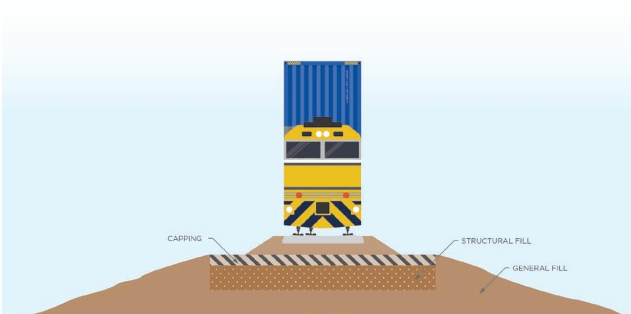
**FIGURE 6.6: STRUCTURE OF THE SUBGRADE**
