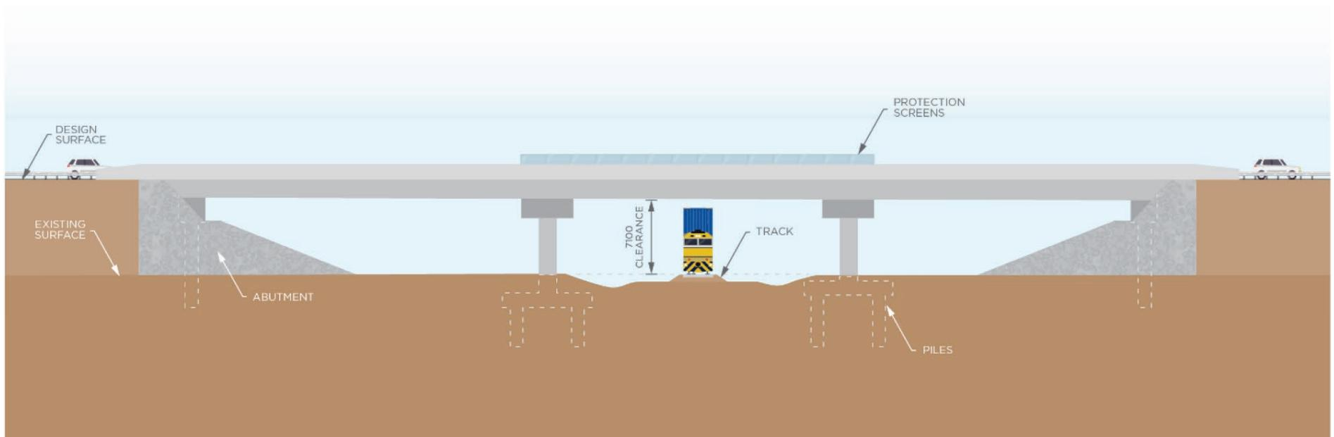
FIGURE 6.12: TYPICAL SECTION OF ROAD OVER RAIL BRIDGE STRUCTURE
