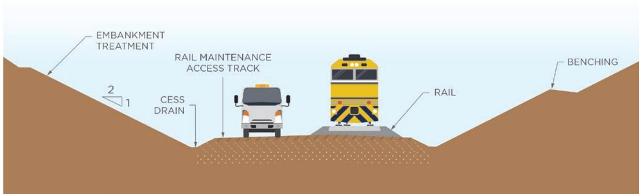
FIGURE 6.16: TYPICAL SECTIONAL DIAGRAM OF RAIL FORMATION SHOWING RAIL MAINTENANCE ACCESS TRACK
