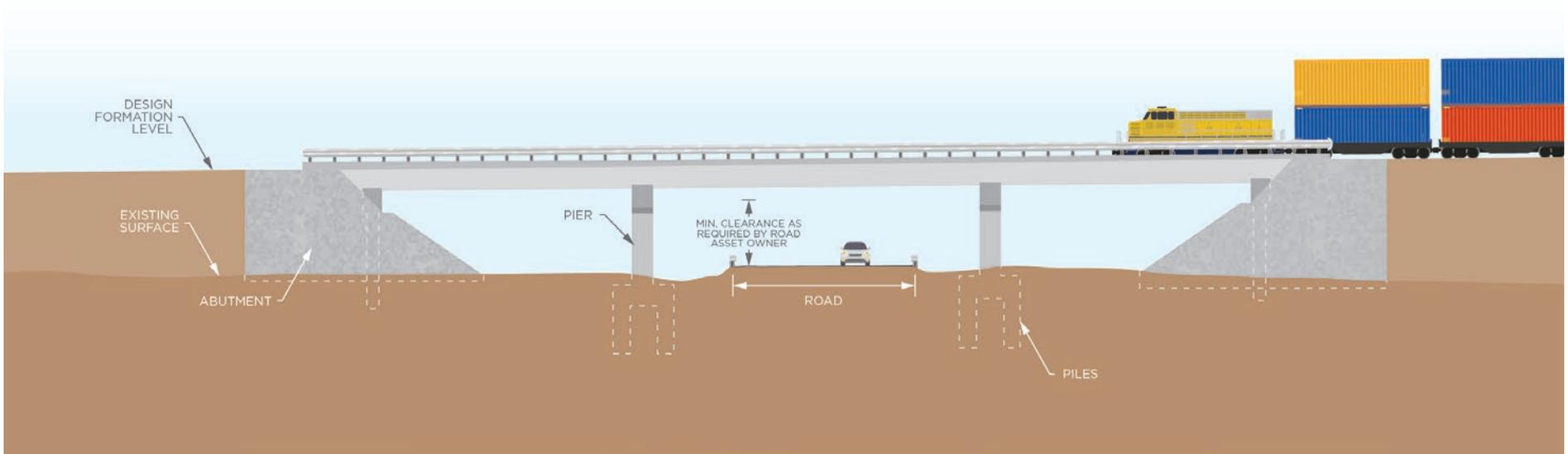
FIGURE 6.11: TYPICAL SECTION OF RAIL OVER ROAD BRIDGE STRUCTURE
