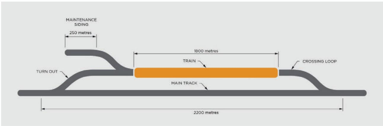
FIGURE 6.7: INDICATIVE DESIGN FOR CROSSING LOOP AND MAINTENANCE SIDING
