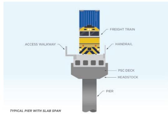
**FIGURE 6.9: TYPICAL PIER WITH PRE-STRESSED CONCRETE SLAB SPAN**
