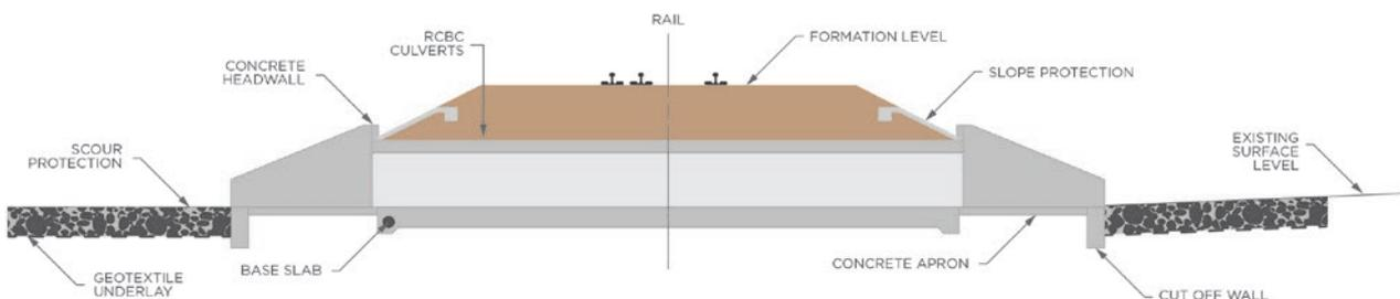
**FIGURE 6: TYPICAL SECTION OF A CROSS-DRAINAGE CULVERT**
