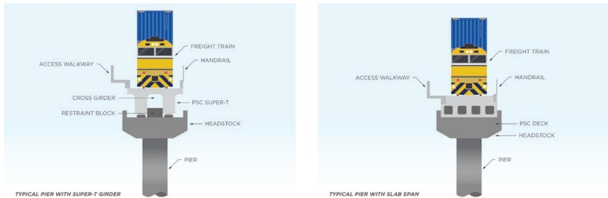
**FIGURE 5: TYPICAL PIER WITH PRE-STRESSED CONCRETE SUPER-T GIRDER (LEFT) AND TYPICAL PIER WITH PRE-STRESSED CONCRETE SLAB SPAN (RIGHT)**
