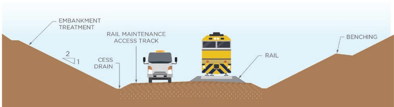
FIGURE 9: TYPICAL SECTIONAL DIAGRAM OF RAIL FORMATION SHOWING A RAIL MAINTENANCE ACCESS TRACK
